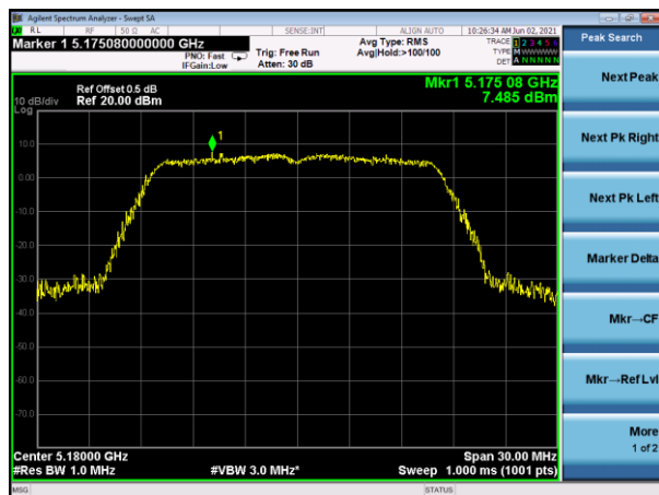
(802.11a) PSD plot on channel 40
