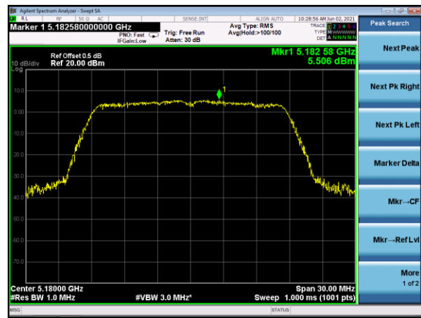
(802.11ac20) PSD plot on channel 40
