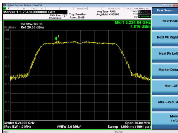
(802.11a) PSD plot on channel 48
