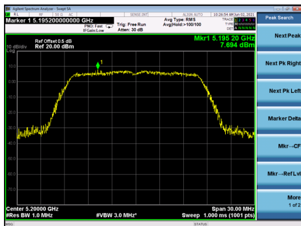
(802.11a) PSD plot on channel 48
