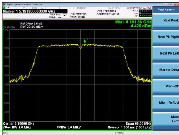
(802.11ac40) PSD plot on channel 46
