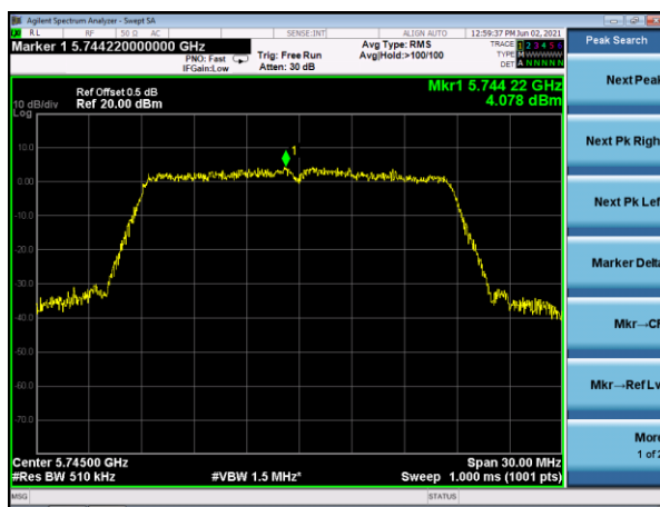
(802.11ac20) PSD plot on channel 157
