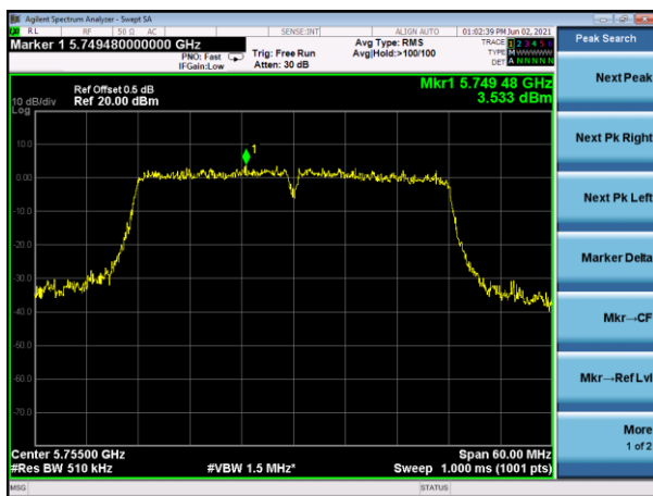
(802.11n40) PSD plot on channel 159
