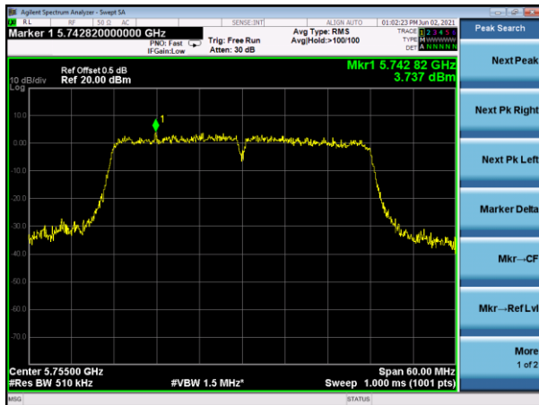
(802.11ac40) PSD plot on channel 159
