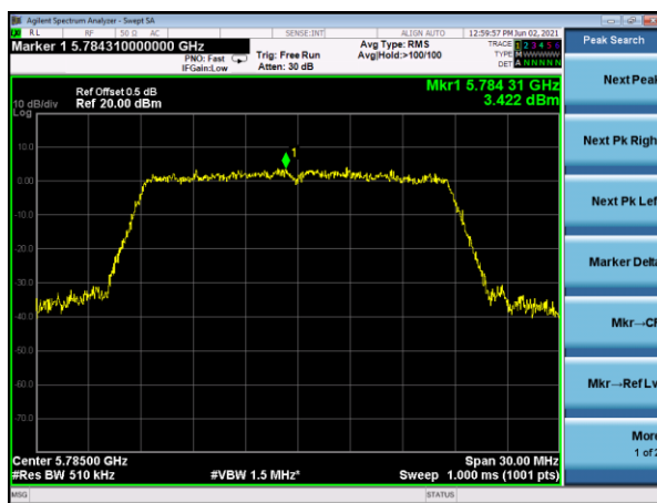
(802.11ac20) PSD plot on channel 165
