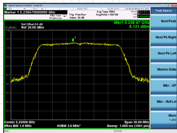
(802.11ac20) PSD plot on channel 48
