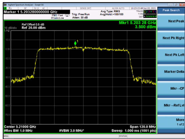
(802.11ac80) PSD plot on channel 42
