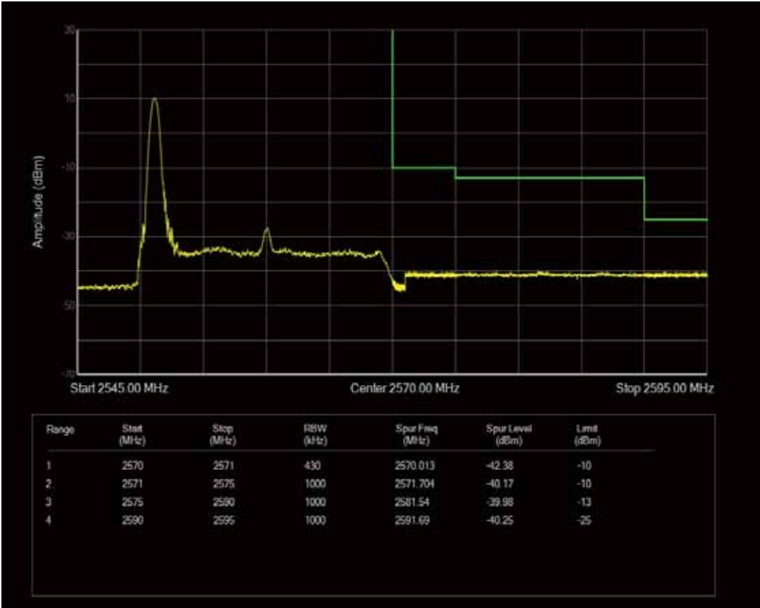
Band7 QAM16 BW=20MHz Channel=21350 RB Size=100 Position=#0
