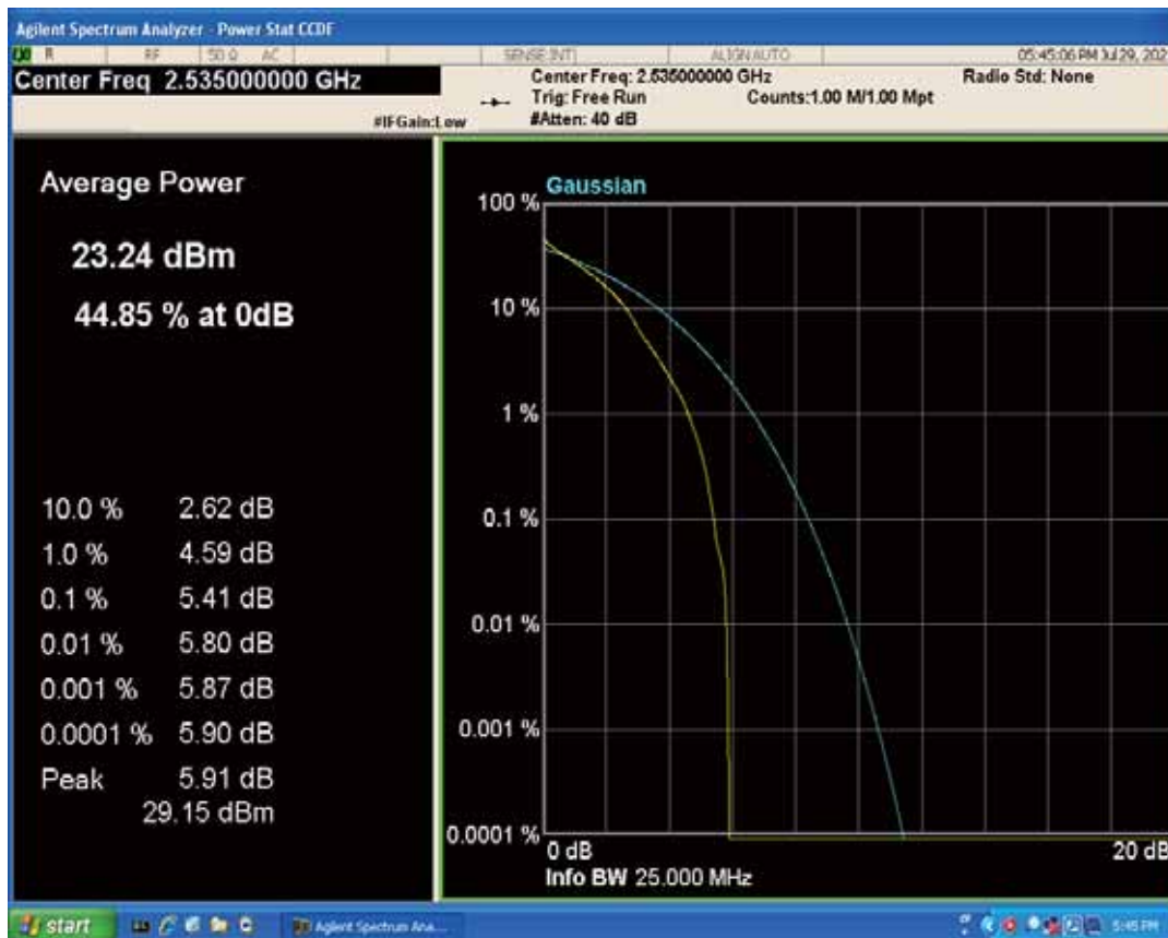
Band7 QAM16 BW=5MHz Channel=21100 RB Size=1 Position=#0
