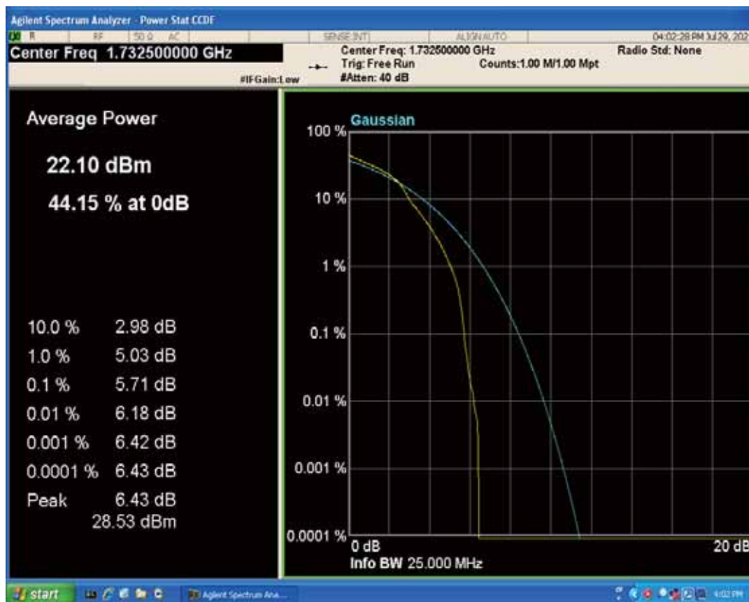
Band4 QAM16 BW=10MHz Channel=20175 RB Size=1 Position=#0
