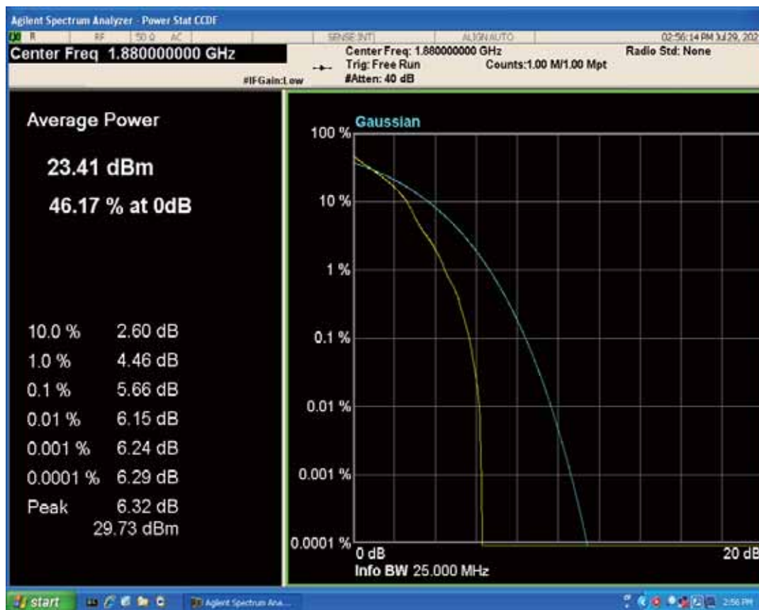
Band2 QAM16 BW=10MHz Channel=18900 RB Size=1 Position=#0
