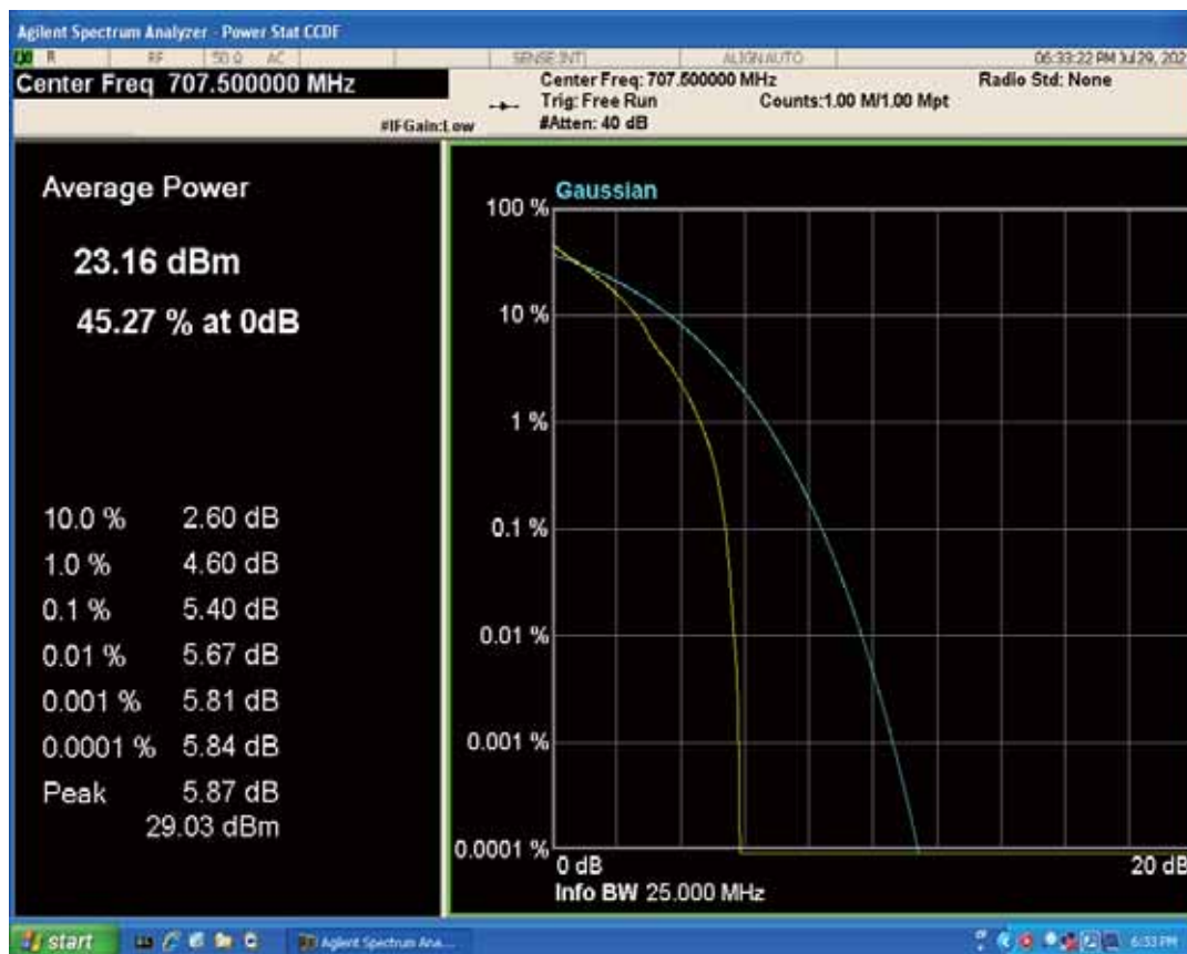
Band12 QAM16 BW=10MHz Channel=23095 RB Size=1 Position=#0
