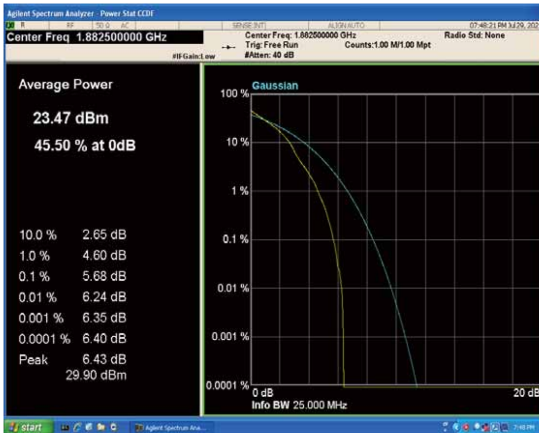
Band25 QAM16 BW=10MHz Channel=26365 RB Size=1 Position=#0
