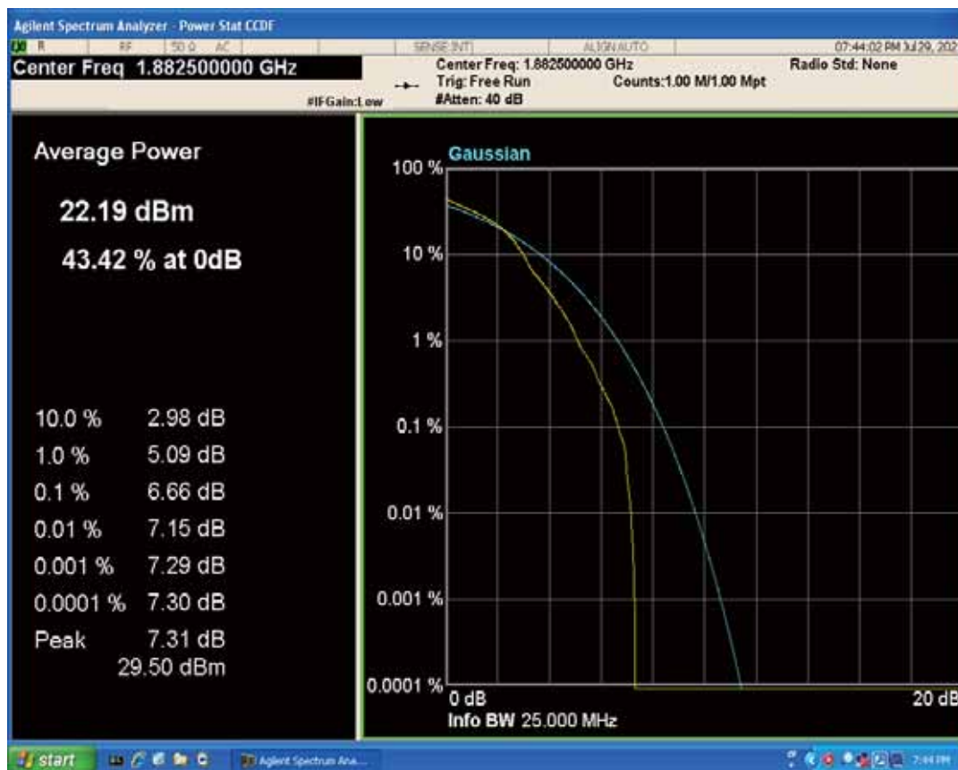
Band25 QAM16 BW=5MHz Channel=26365 RB Size=1 Position=#0
