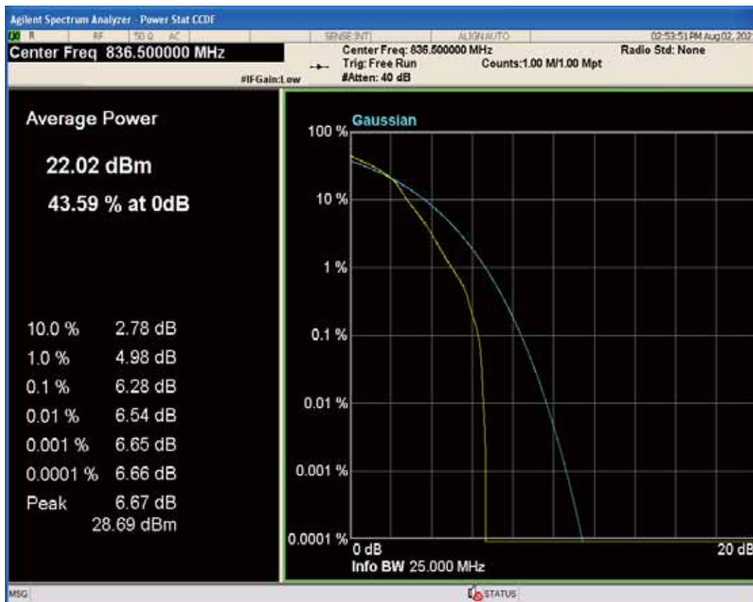
Band26b QAM16 BW=10MHz Channel=26915 RB Size=1 Position=#0
