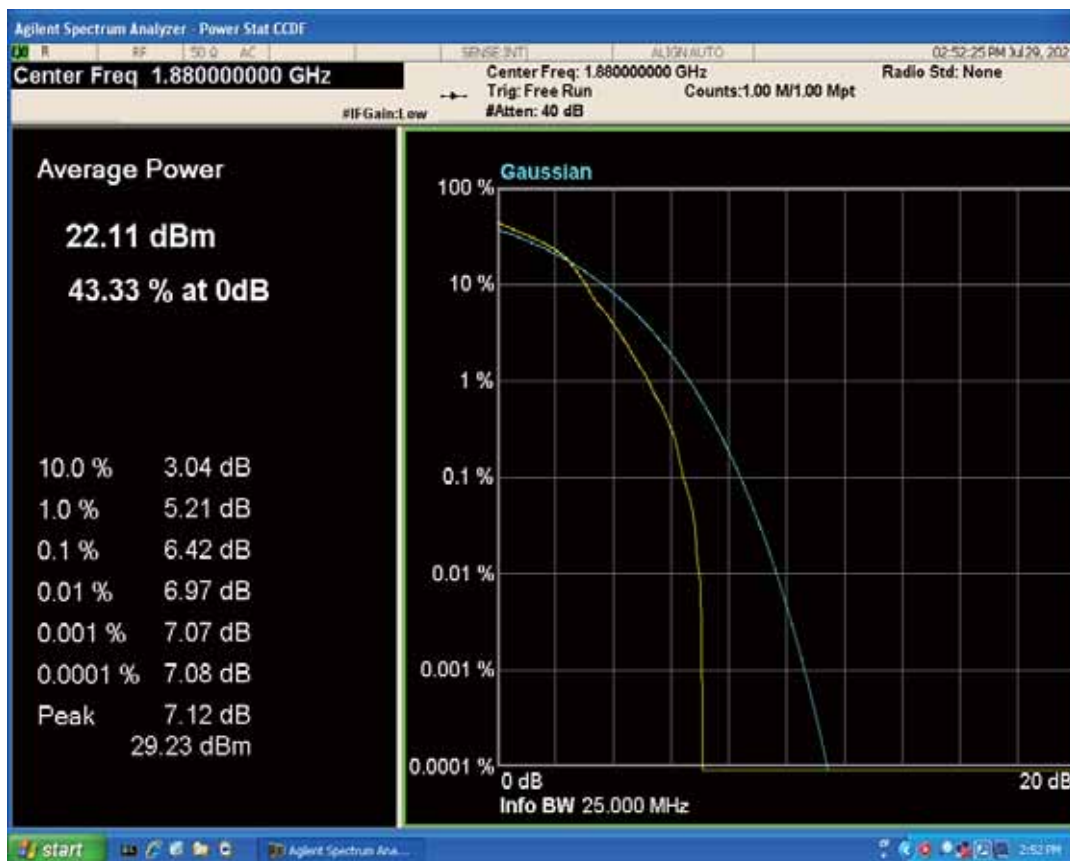
Band2 QAM16 BW=3MHz Channel=18900 RB Size=1 Position=#0
