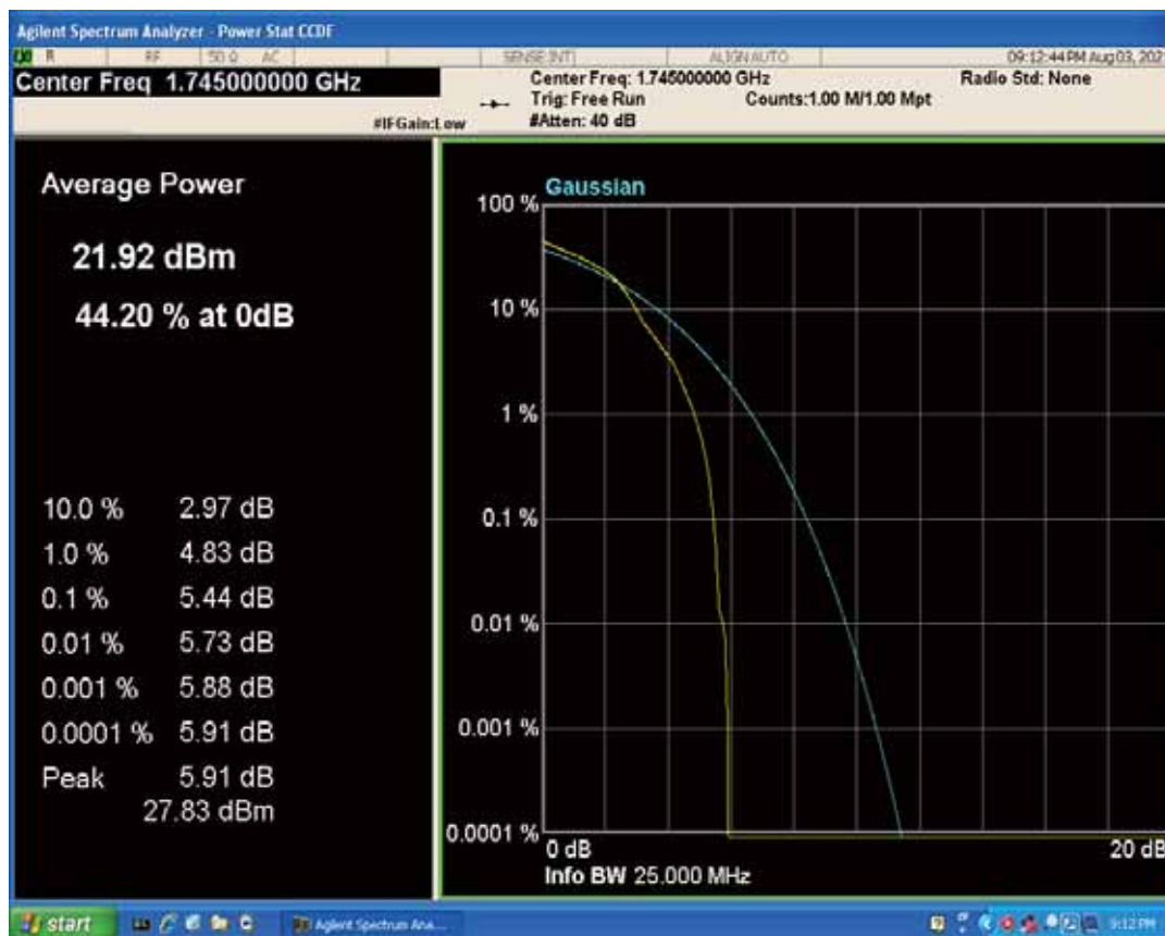
Band66 QPSK BW=3MHz Channel=132322 RB Size=1 Position=#0
