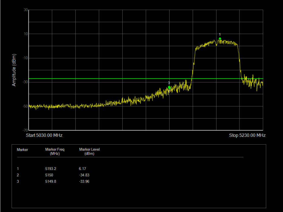
Band Edge NVNT 802.11ac40 5190MHz Low Ant1
