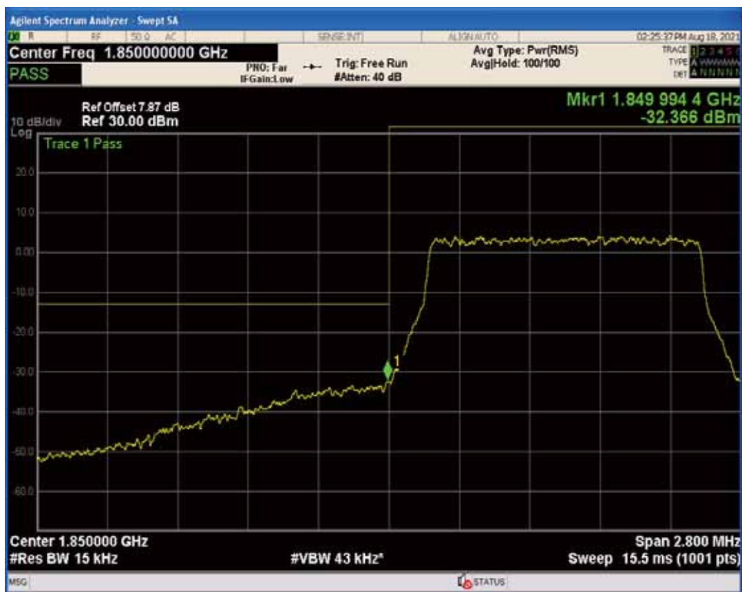
Band25 QPSK BW=1.4MHz Channel=26683 RB Size=1 Position=#Max
