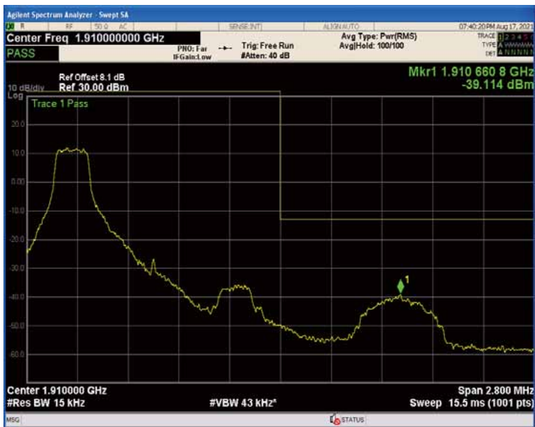
Band2 QPSK BW=1.4MHz Channel=19193 RB Size=1 Position=#Max
