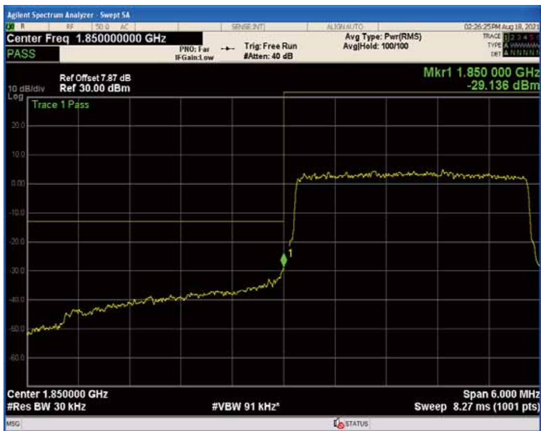
Band25 QAM16 BW=3MHz Channel=26055 RB Size=1 Position=#0
