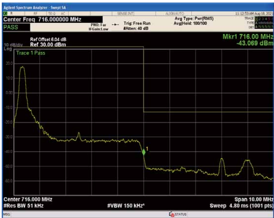
Band17 QPSK BW=5MHz Channel=23825 RB Size=1 Position=#Max
