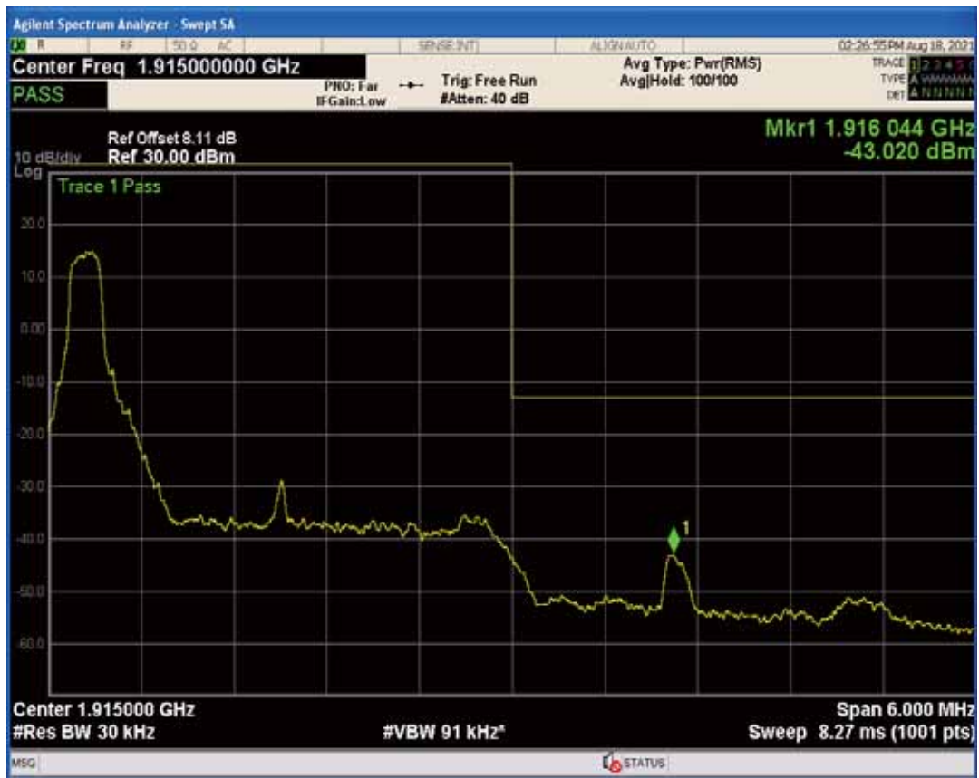
Band25 QAM16 BW=3MHz Channel=26675 RB Size=1 Position=#Max
