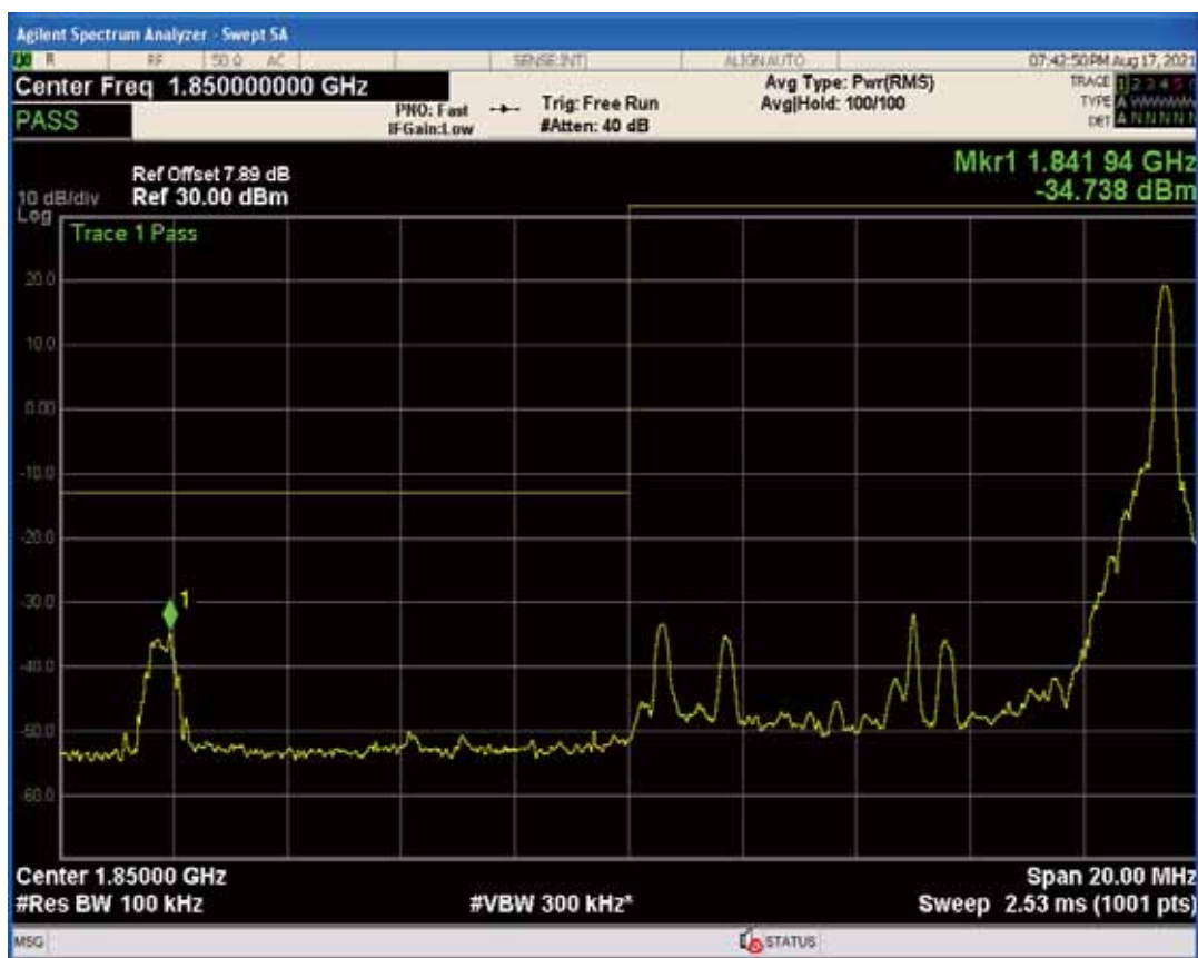
Band2 QPSK BW=10MHz Channel=18650 RB Size=50 Position=#0
