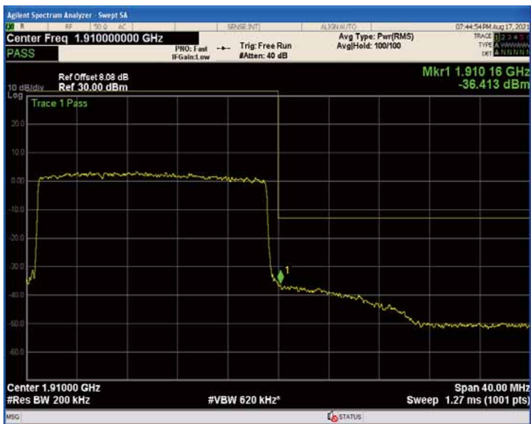
Band2 QAM16 BW=20MHz Channel=19100 RB Size=1 Position=#Max
