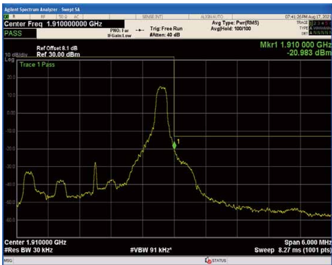
Band2 QPSK BW=3MHz Channel=19185 RB Size=15 Position=#0
