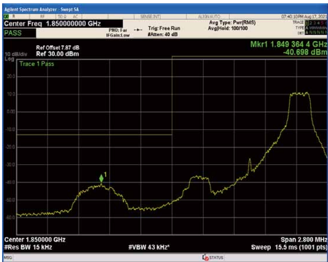
Band2 QPSK BW=1.4MHz Channel=19193 RB Size=1 Position=#0
