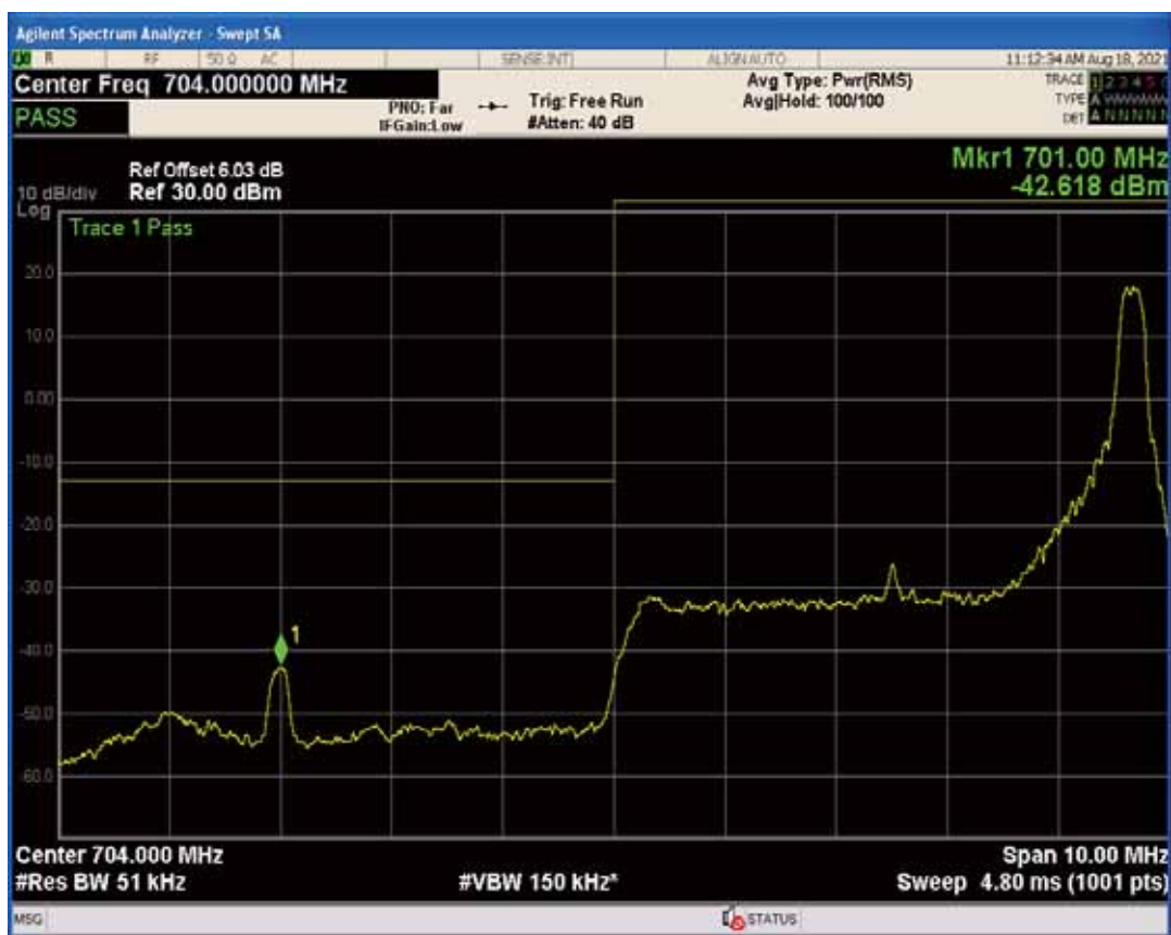
Band17 QPSK BW=5MHz Channel=23755 RB Size=25 Position=#0
