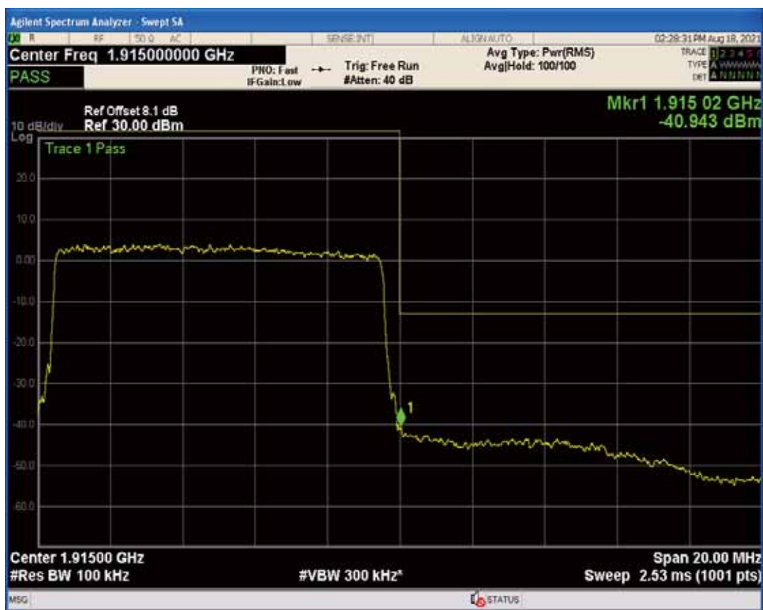
Band25 QPSK BW=10MHz Channel=26640 RB Size=1 Position=#Max
