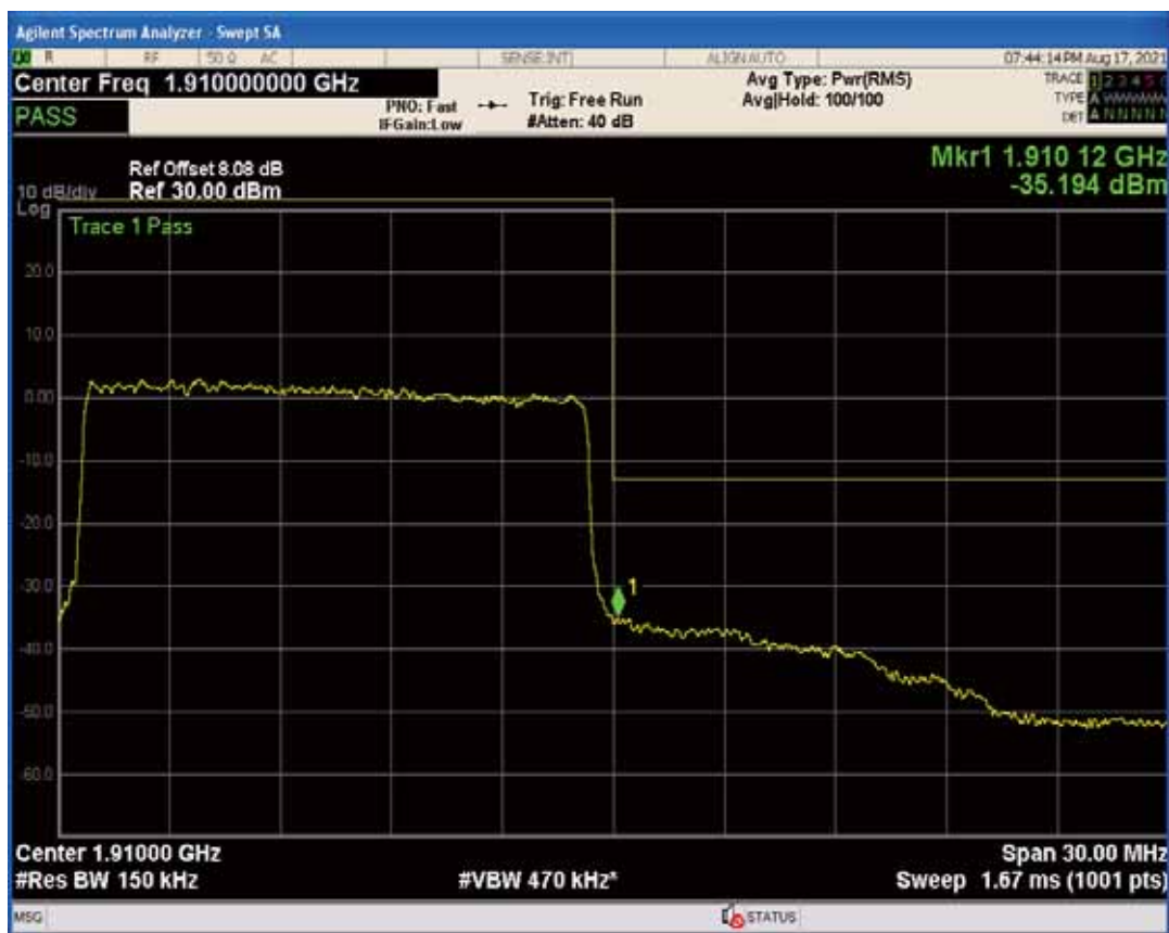
Band2 QPSK BW=20MHz Channel=18700 RB Size=1 Position=#Max
