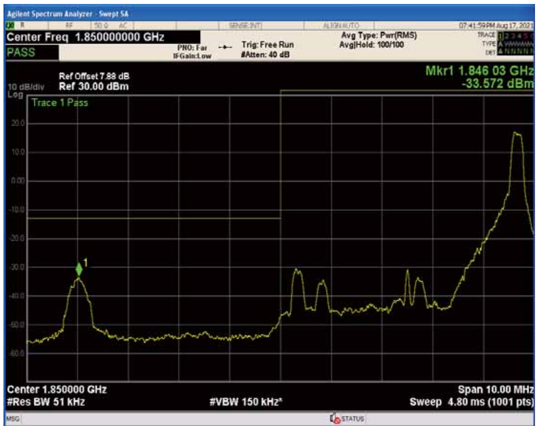
Band2 QPSK BW=5MHz Channel=18625 RB Size=1 Position=#0
