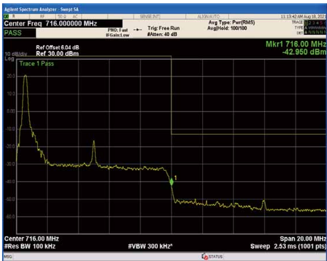
Band17 QPSK BW=10MHz Channel=23800 RB Size=50 Position=#0
