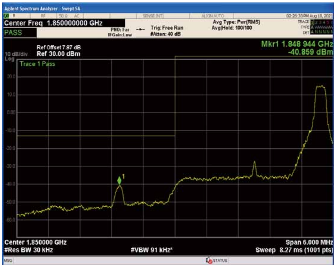
Band25 QAM16 BW=3MHz Channel=26055 RB Size=15 Position=#0
