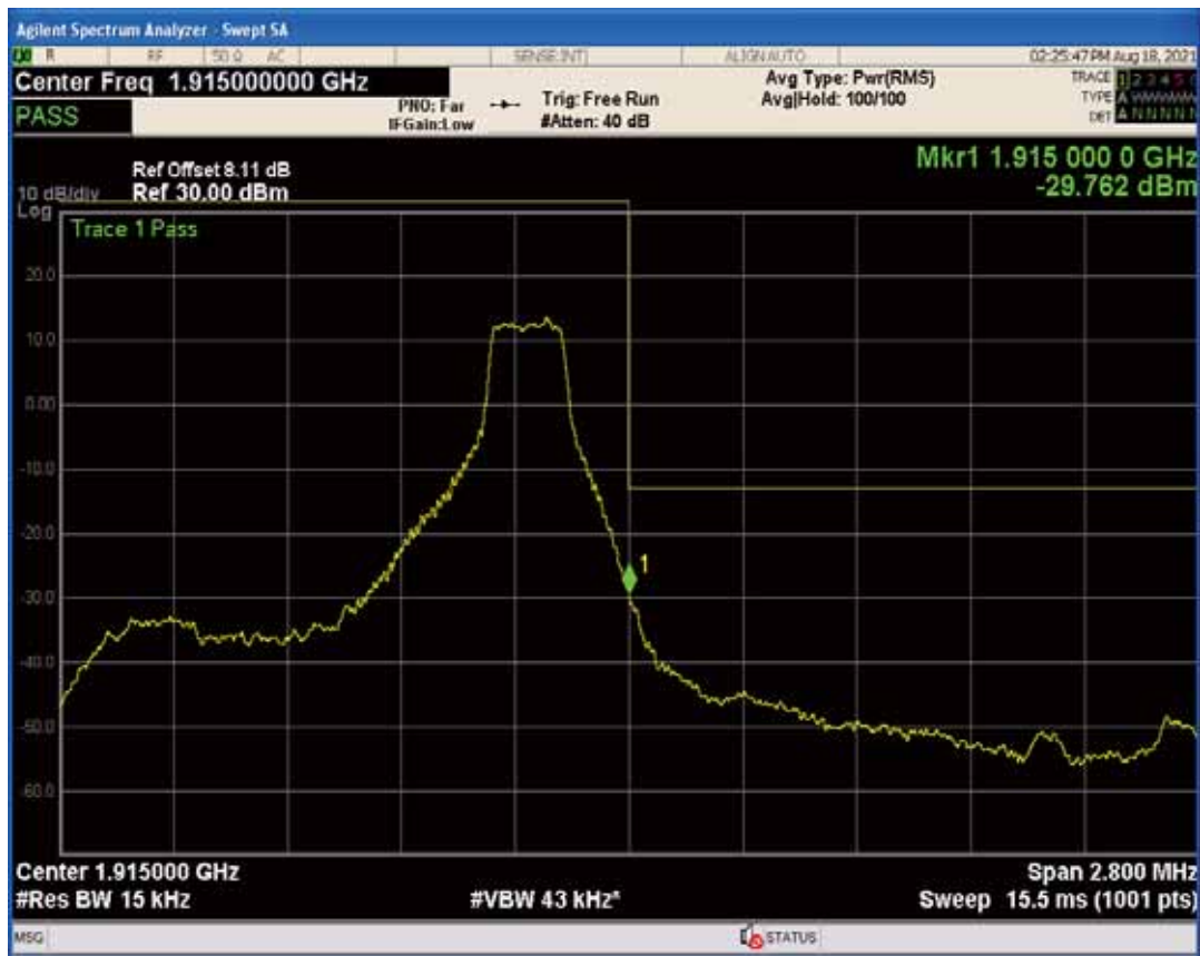
Band25 QPSK BW=1.4MHz Channel=26683 RB Size=6 Position=#0
