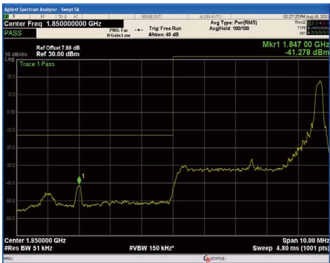
Band25 QAM16 BW=5MHz Channel=26065 RB Size=1 Position=#0
