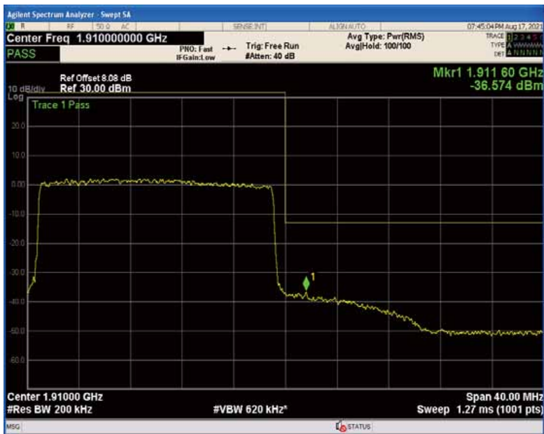
Band25 QPSK BW=1.4MHz Channel=26047 RB Size=1 Position=#Max
