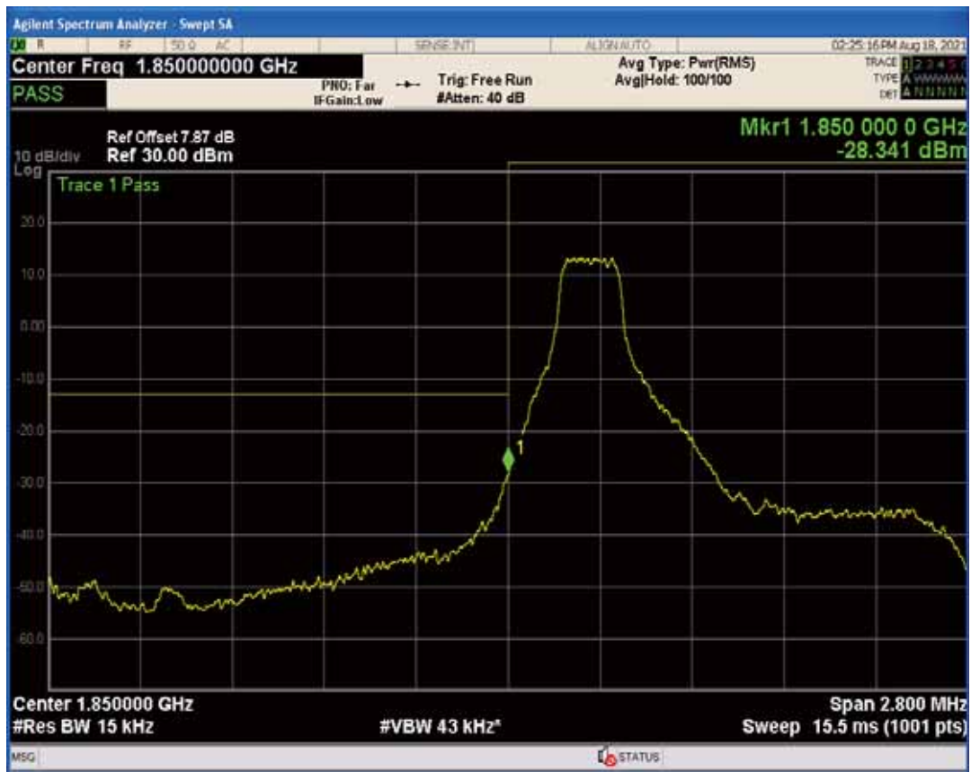
Band25 QAM16 BW=1.4MHz Channel=26047 RB Size=1 Position=#0
