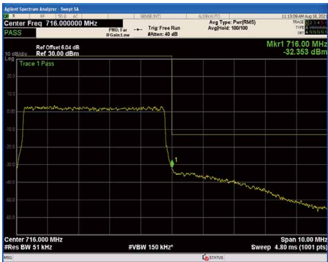
Band17 QAM16 BW=5MHz Channel=23825 RB Size=1 Position=#Max
