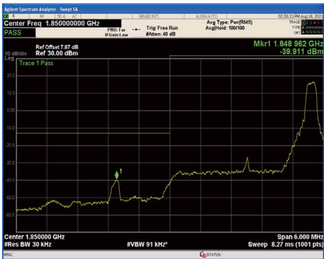
Band25 QPSK BW=3MHz Channel=26055 RB Size=15 Position=#0
