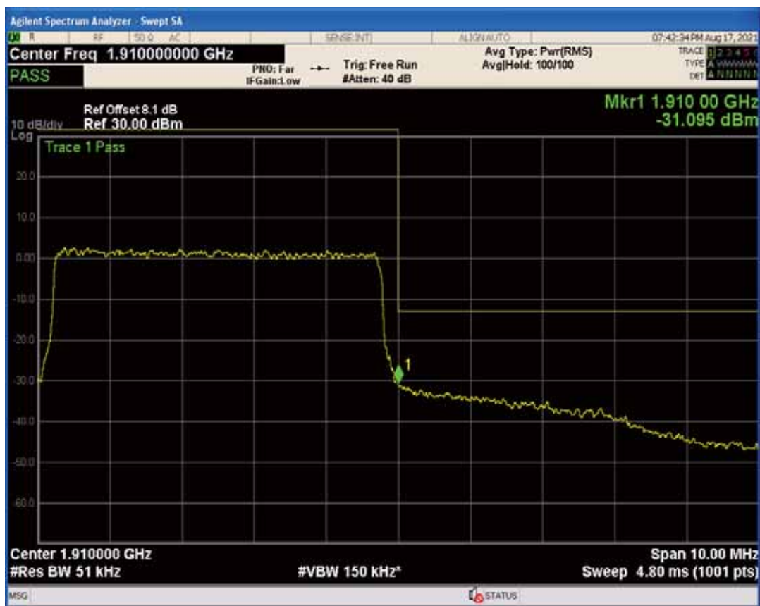
Band2 QAM16 BW=5MHz Channel=19175 RB Size=1 Position=#Max
