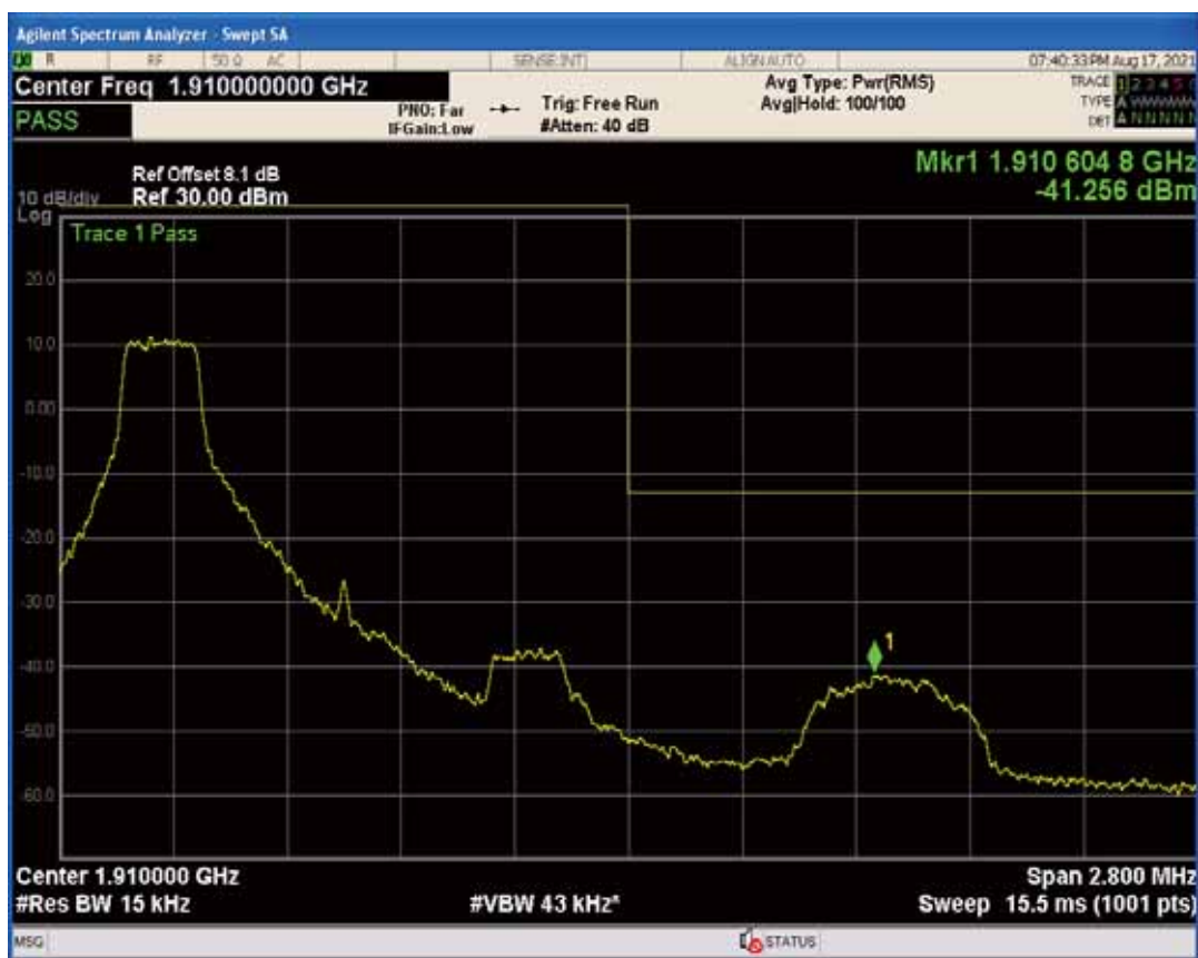
Band2 QAM16 BW=1.4MHz Channel=19193 RB Size=6 Position=#0
