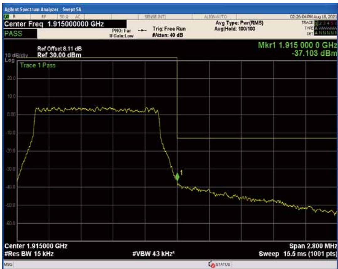
Band25 QPSK BW=3MHz Channel=26055 RB Size=1 Position=#Max
