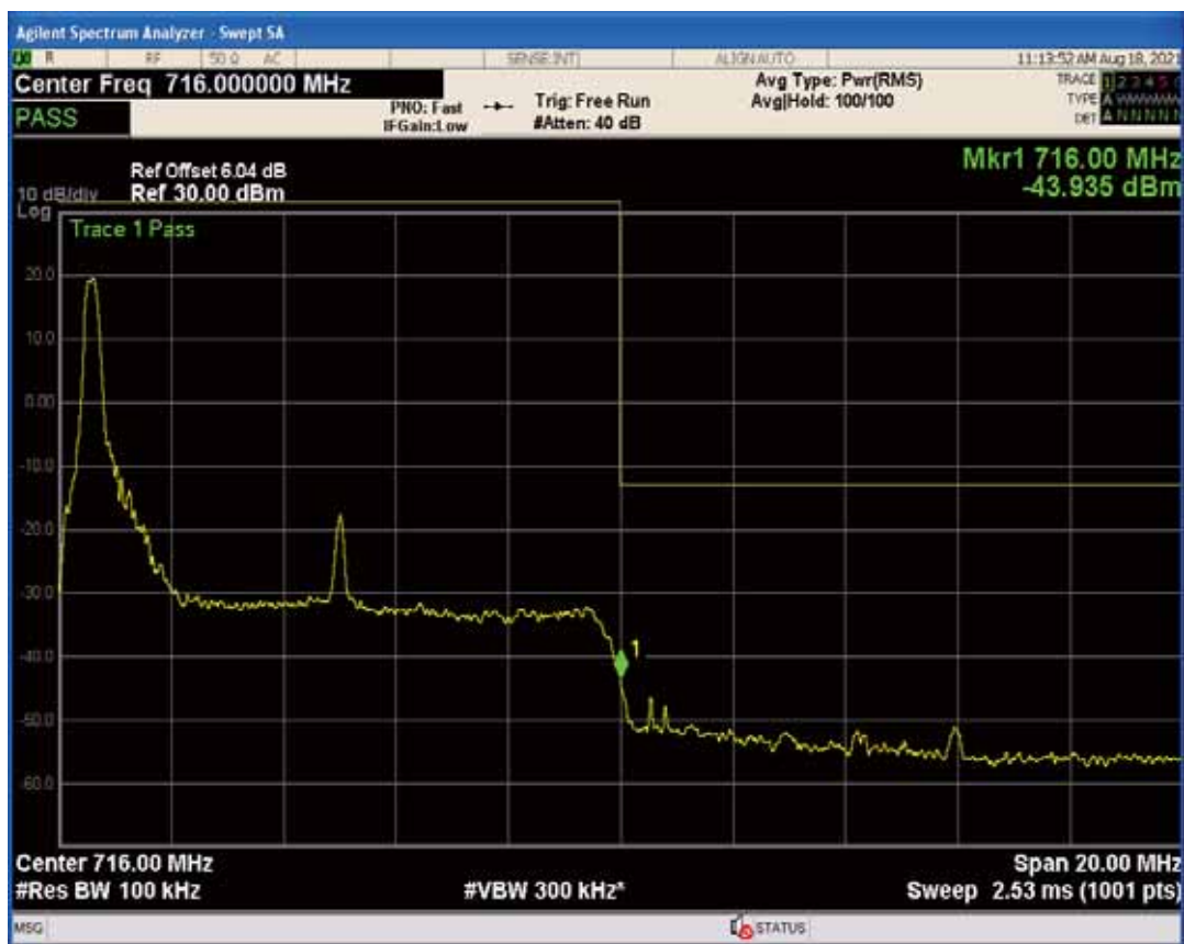
Band17 QAM16 BW=10MHz Channel=23800 RB Size=50 Position=#0
