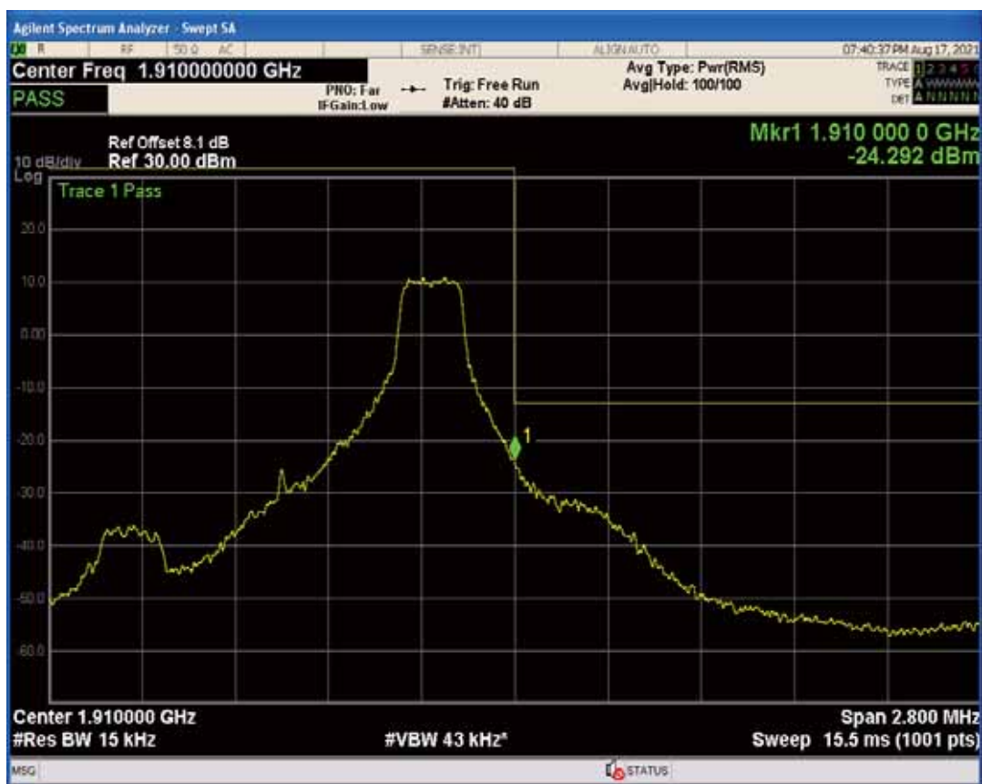
Band2 QPSK BW=3MHz Channel=18615 RB Size=1 Position=#Max
