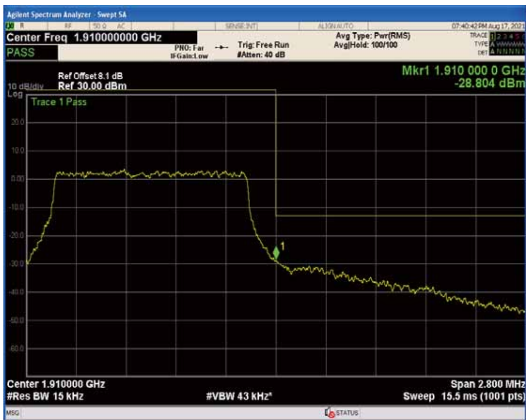
Band2 QAM16 BW=1.4MHz Channel=19193 RB Size=1 Position=#Max
