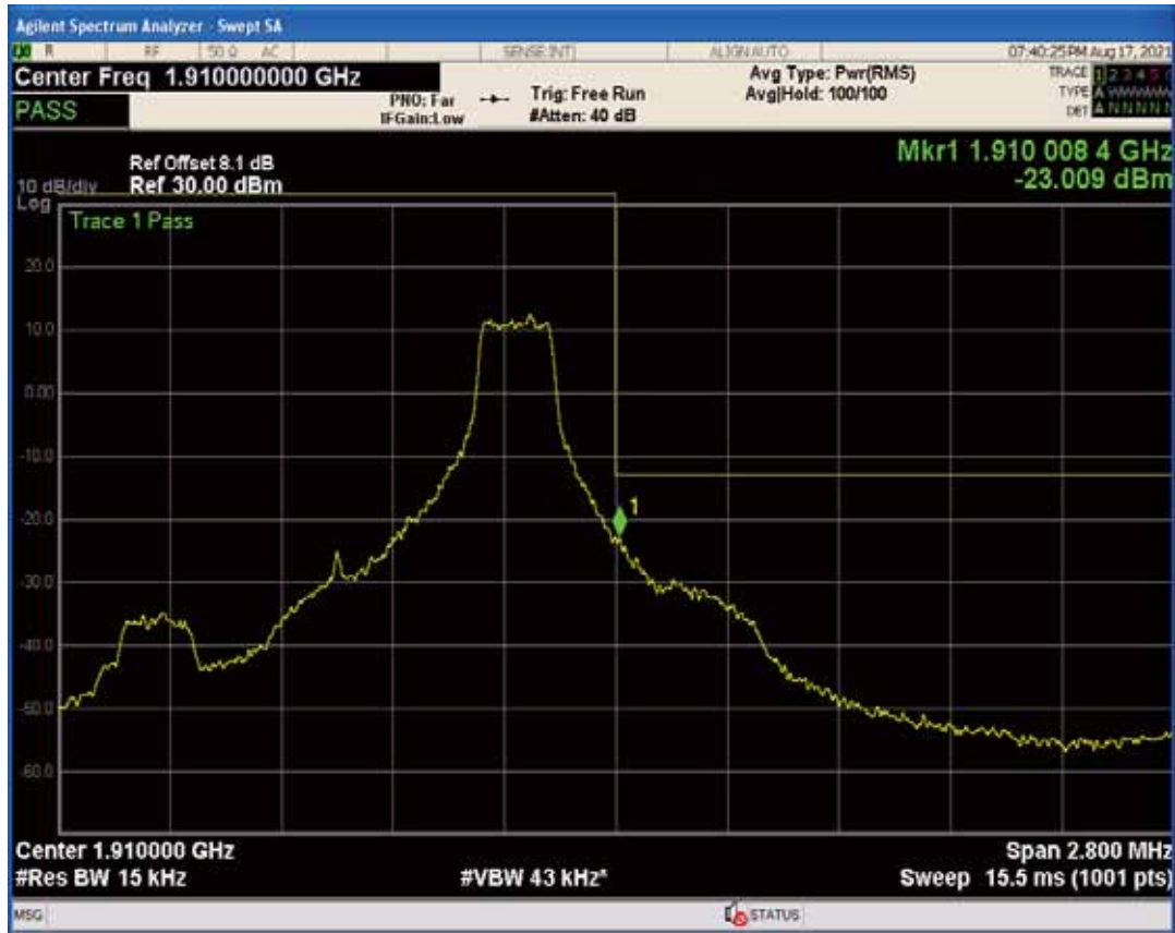
Band2 QPSK BW=1.4MHz Channel=19193 RB Size=6 Position=#0
