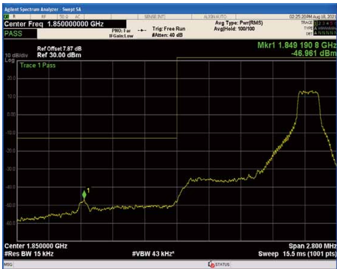
Band25 QPSK BW=1.4MHz Channel=26047 RB Size=1 Position=#0
