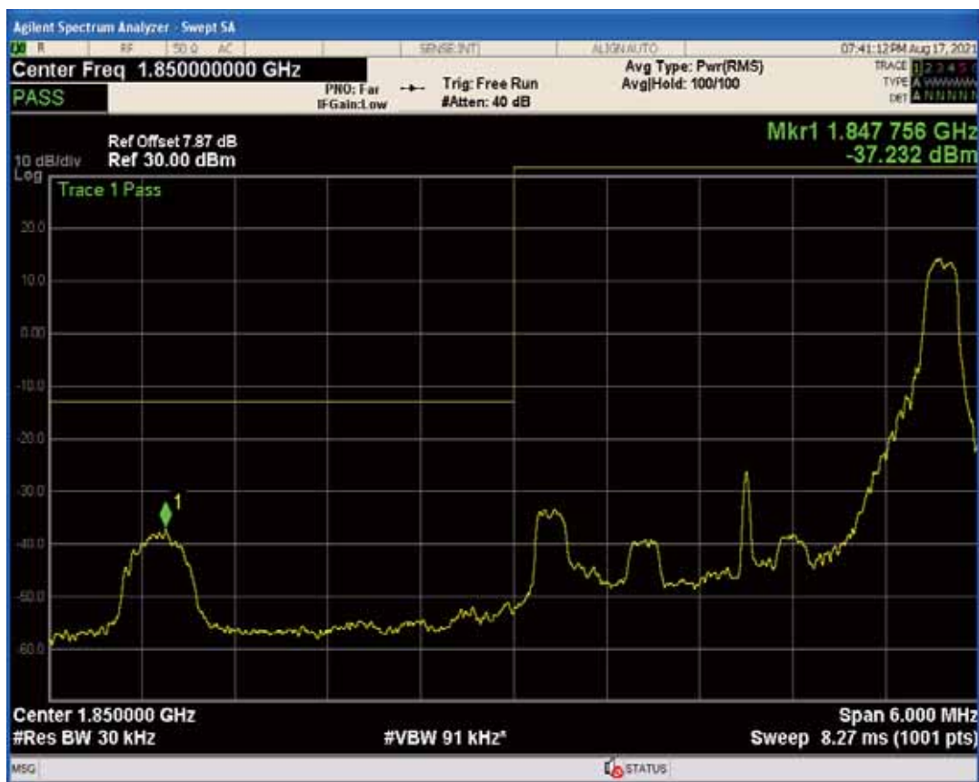
Band2 QAM16 BW=3MHz Channel=18615 RB Size=15 Position=#0
