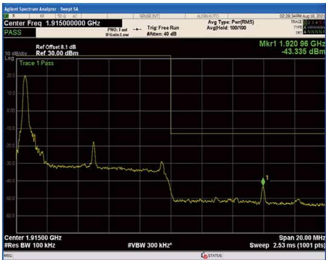
Band25 QAM16 BW=10MHz Channel=26640 RB Size=50 Position=#0
