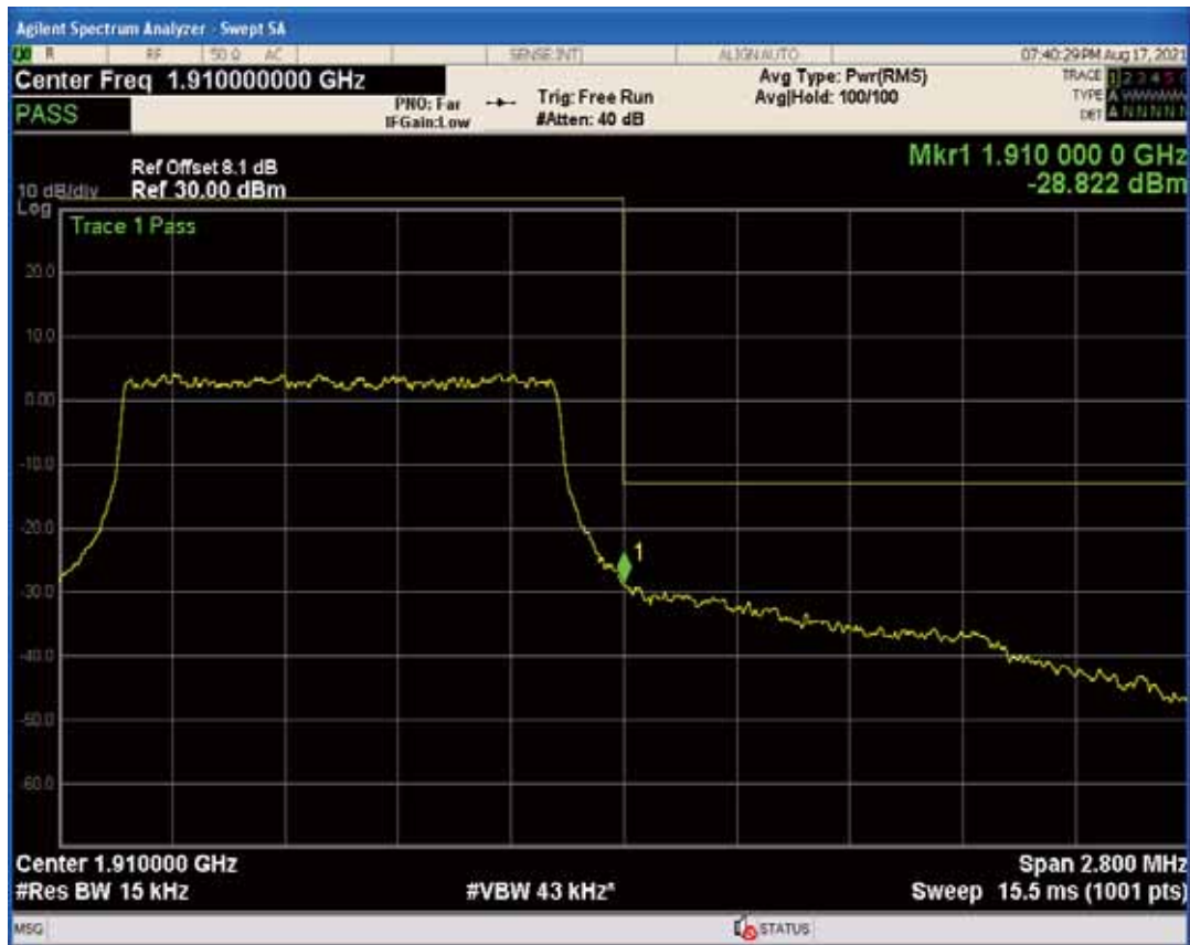
Band2 QAM16 BW=1.4MHz Channel=19193 RB Size=1 Position=#0
