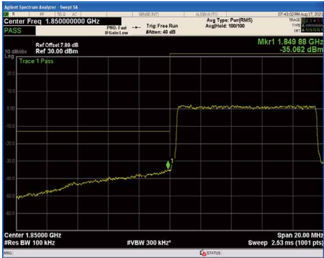
Band2 QPSK BW=10MHz Channel=19150 RB Size=1 Position=#0
