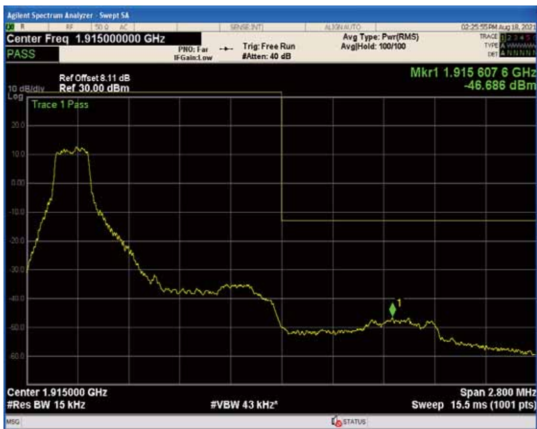
Band25 QAM16 BW=1.4MHz Channel=26683 RB Size=1 Position=#Max
