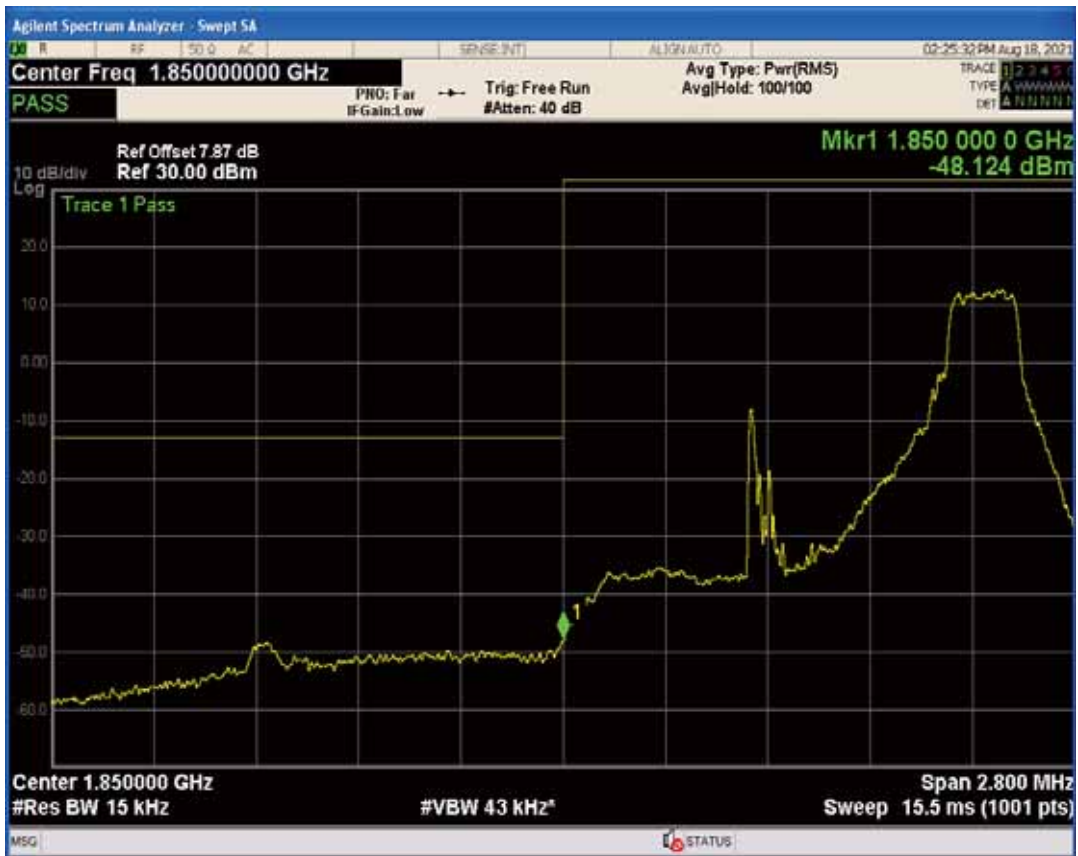
Band25 QPSK BW=1.4MHz Channel=26683 RB Size=1 Position=#0
