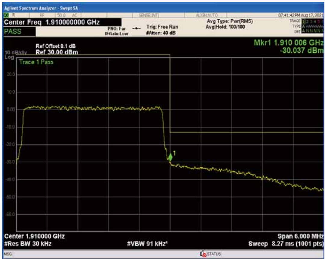
Band2 QPSK BW=5MHz Channel=18625 RB Size=1 Position=#Max
