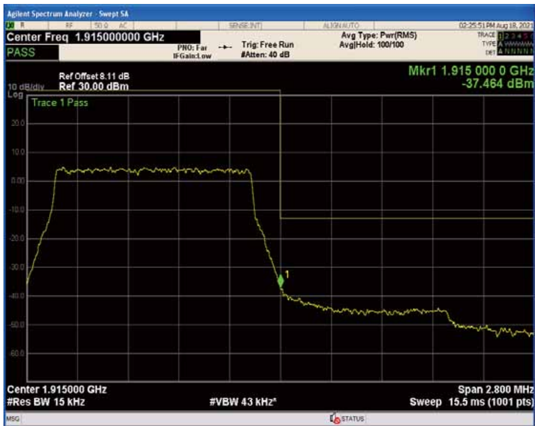
Band25 QAM16 BW=1.4MHz Channel=26683 RB Size=1 Position=#0
