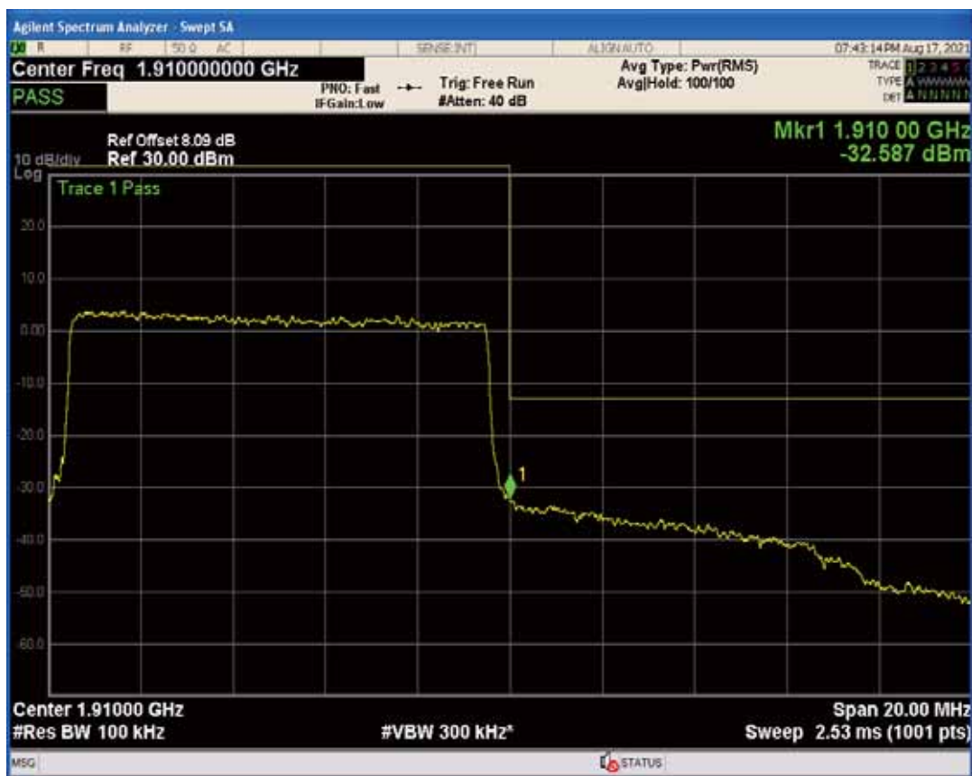
Band2 QAM16 BW=10MHz Channel=19150 RB Size=1 Position=#0
