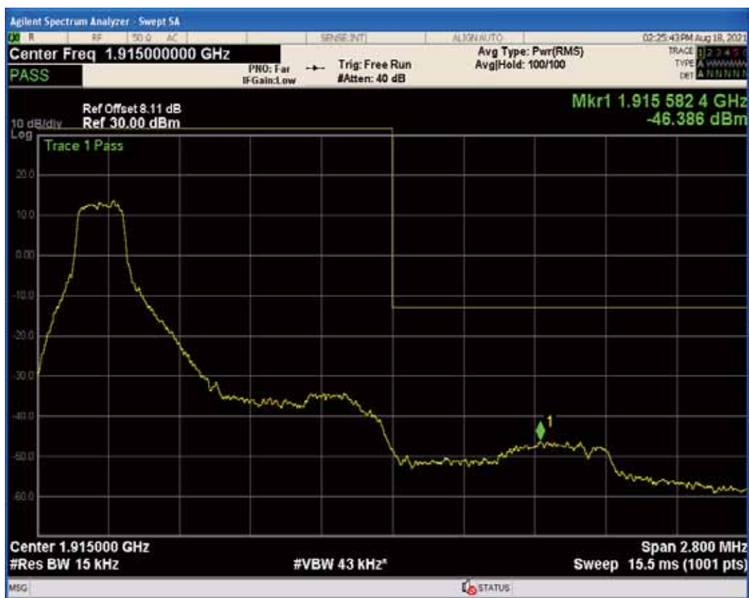
Band25 QAM16 BW=1.4MHz Channel=26047 RB Size=6 Position=#0
