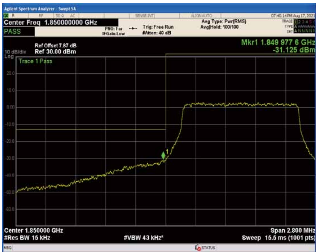
Band2 QAM16 BW=1.4MHz Channel=18607 RB Size=1 Position=#Max
