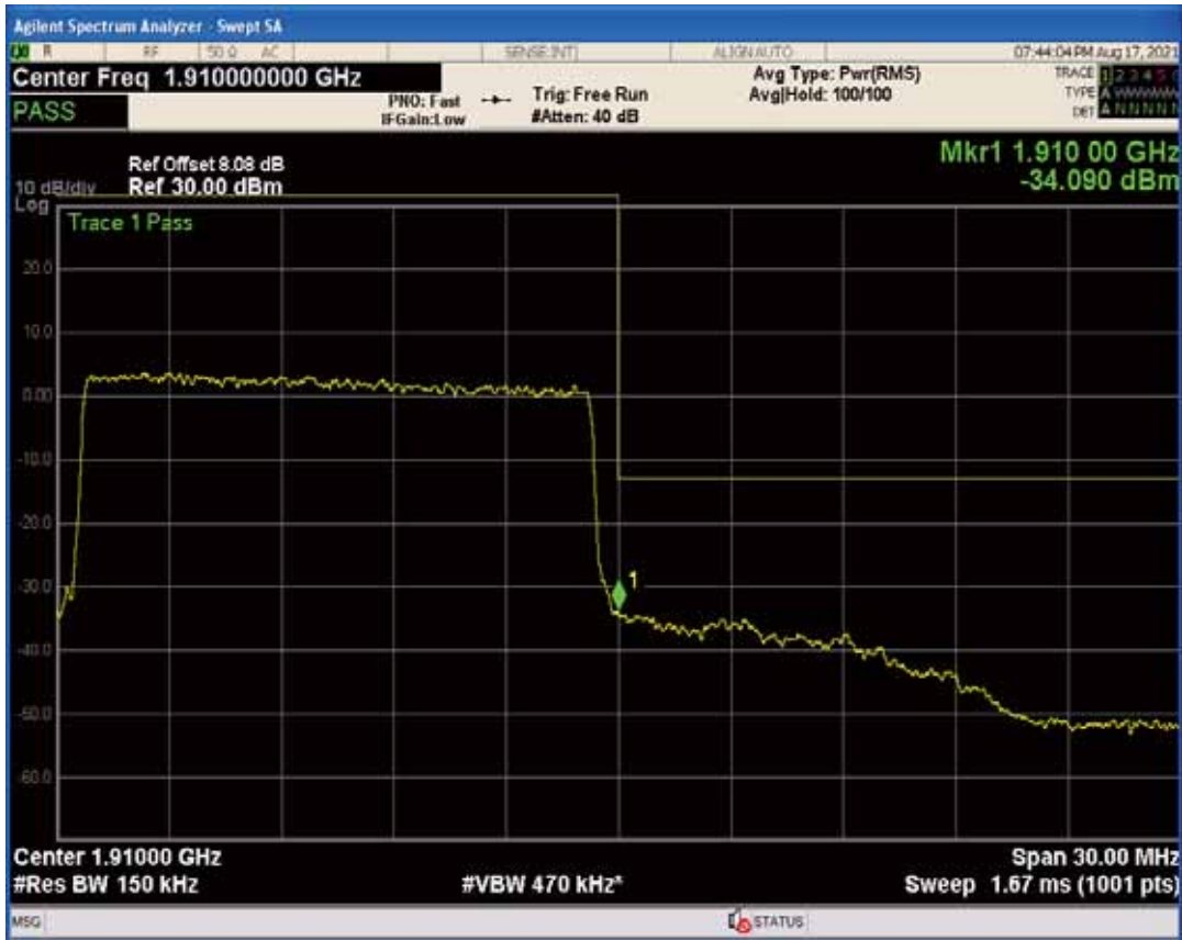
Band2 QAM16 BW=15MHz Channel=19125 RB Size=1 Position=#Max
