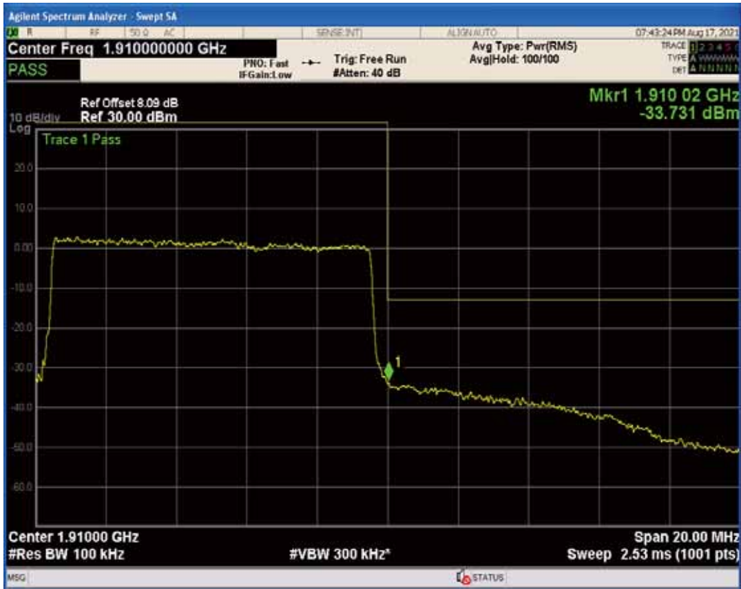
Band2 QPSK BW=15MHz Channel=18675 RB Size=1 Position=#Max
