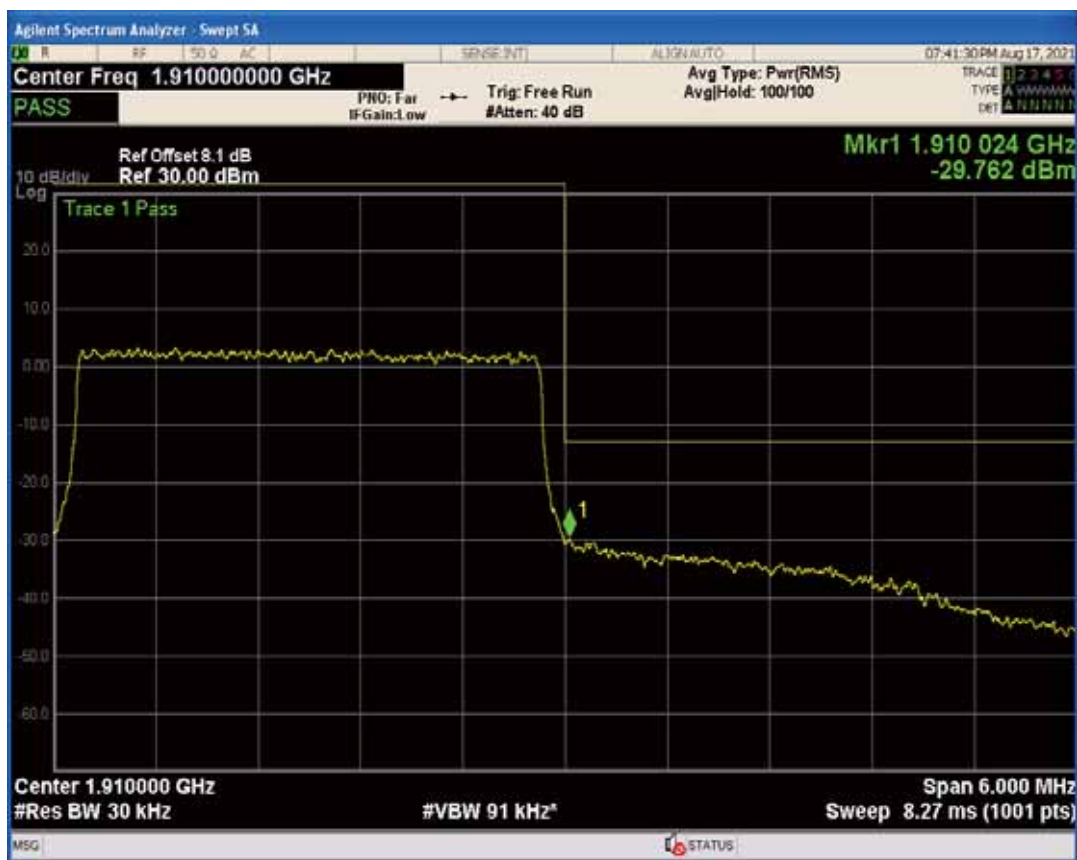
Band2 QAM16 BW=3MHz Channel=19185 RB Size=1 Position=#0
