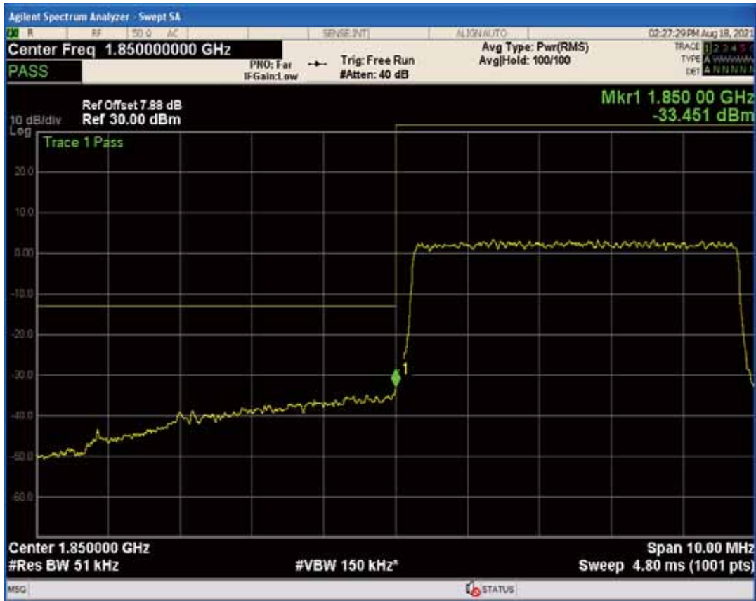
Band25 QPSK BW=5MHz Channel=26665 RB Size=1 Position=#0
