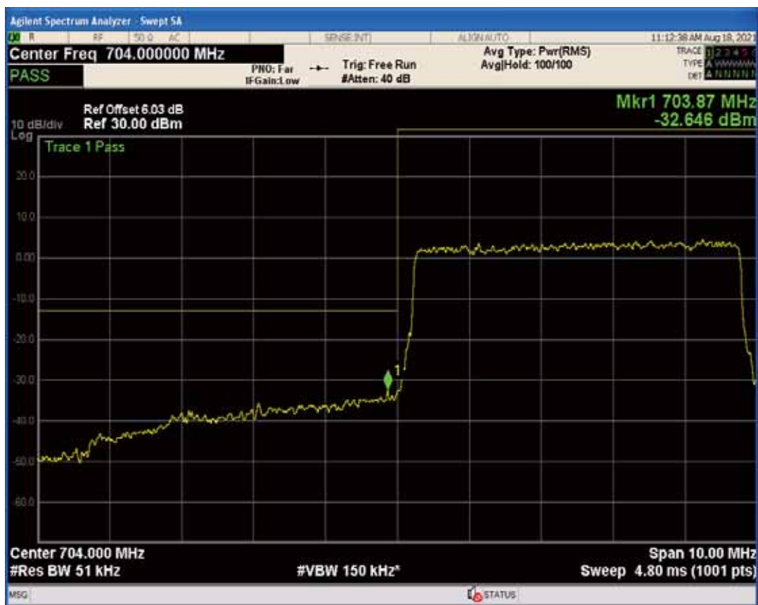
Band17 QAM16 BW=5MHz Channel=23755 RB Size=1 Position=#0
