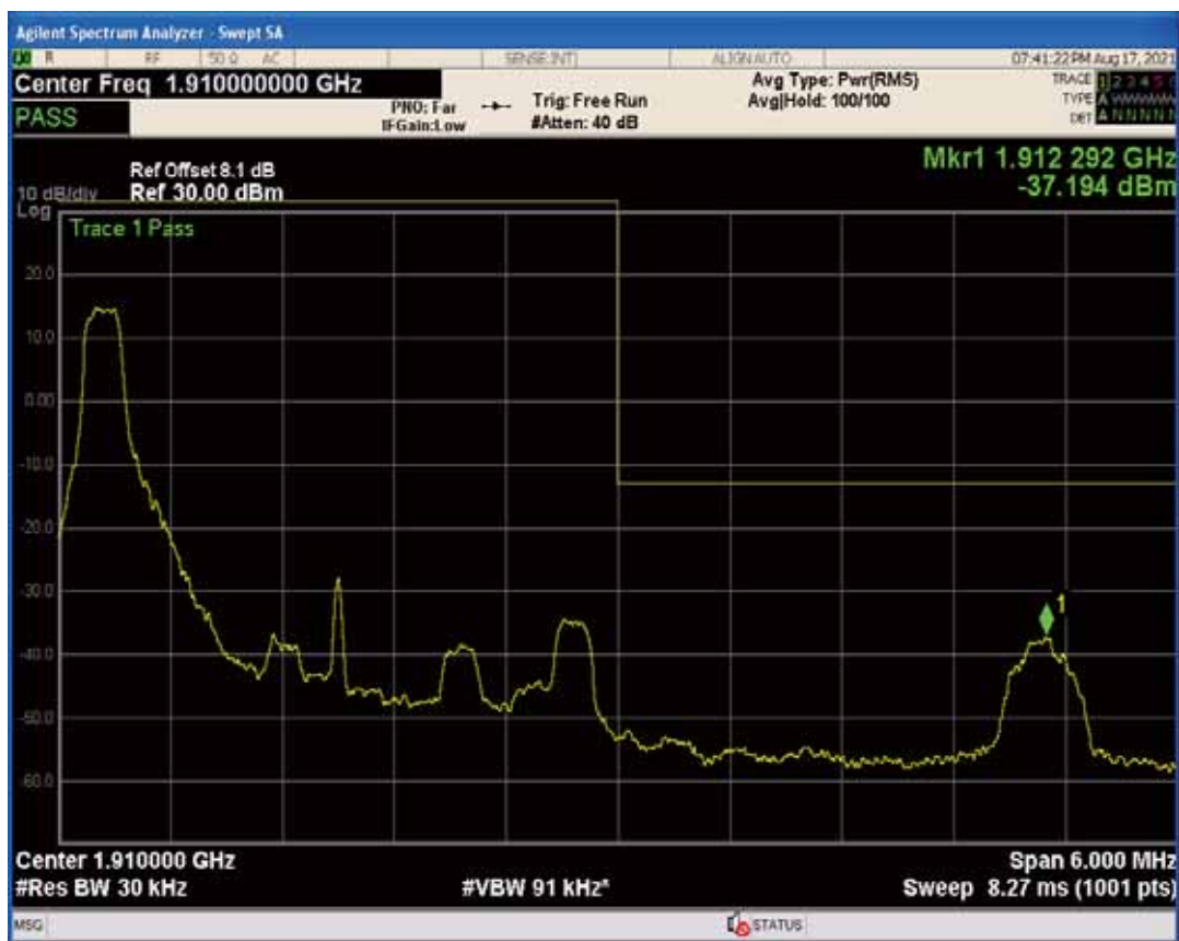
Band2 QPSK BW=3MHz Channel=19185 RB Size=1 Position=#Max
