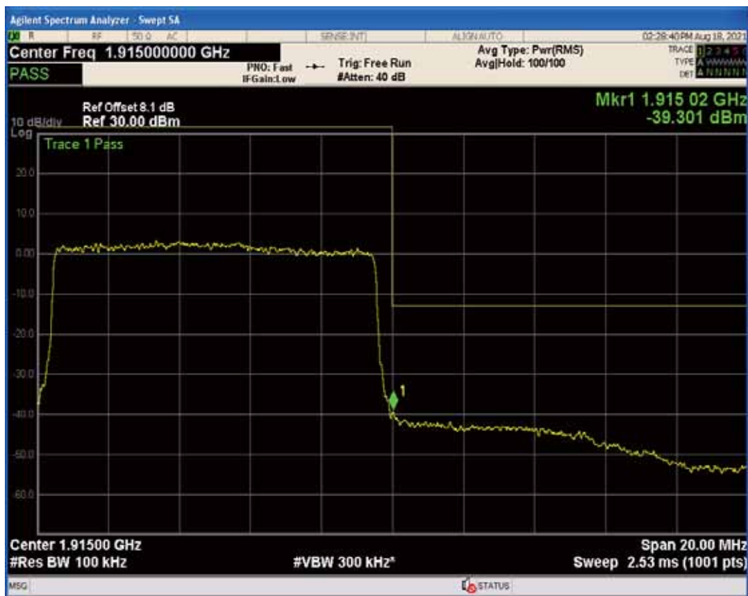
Band25 QPSK BW=15MHz Channel=26115 RB Size=1 Position=#0
