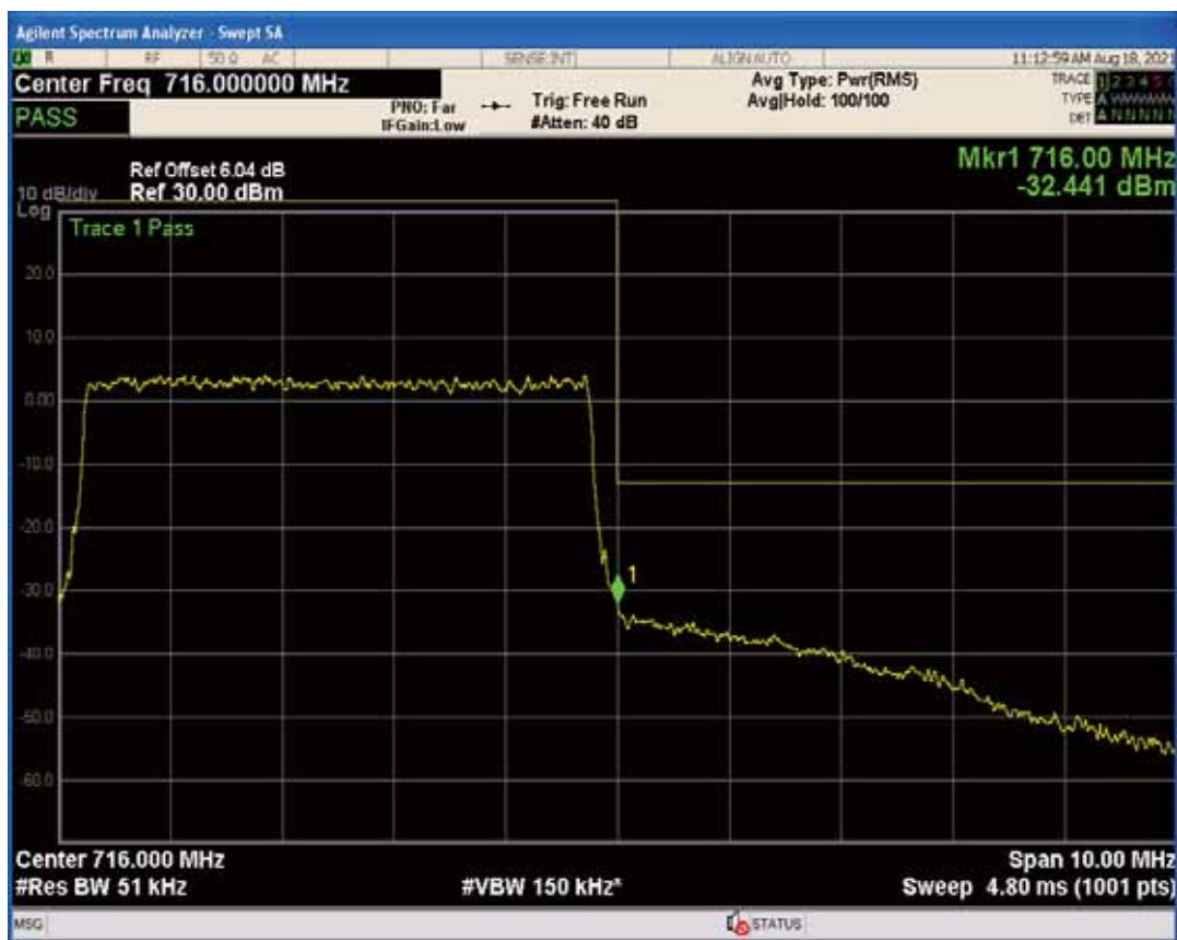
Band17 QAM16 BW=5MHz Channel=23825 RB Size=1 Position=#0
