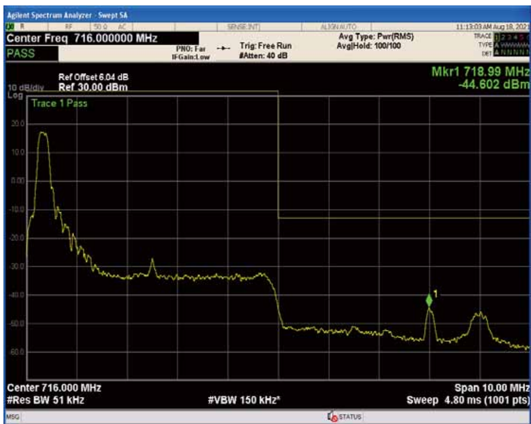
Band17 QAM16 BW=5MHz Channel=23825 RB Size=25 Position=#0
