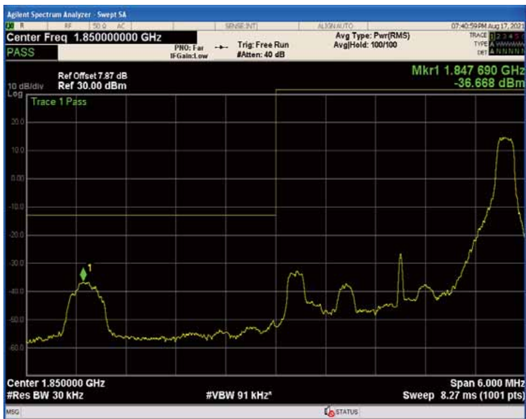
Band2 QPSK BW=3MHz Channel=18615 RB Size=1 Position=#0
