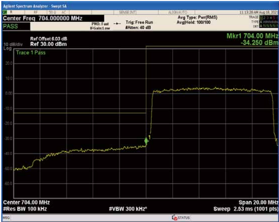
Band17 QPSK BW=10MHz Channel=23780 RB Size=1 Position=#Max
