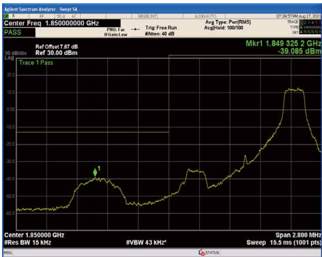
Band2 QPSK BW=1.4MHz Channel=18607 RB Size=6 Position=#0
