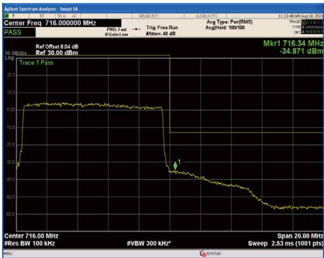
Band17 QAM16 BW=10MHz Channel=23800 RB Size=1 Position=#Max
