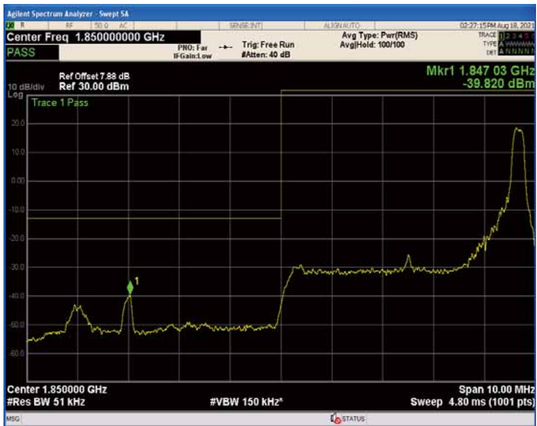
Band25 QPSK BW=5MHz Channel=26065 RB Size=1 Position=#0
