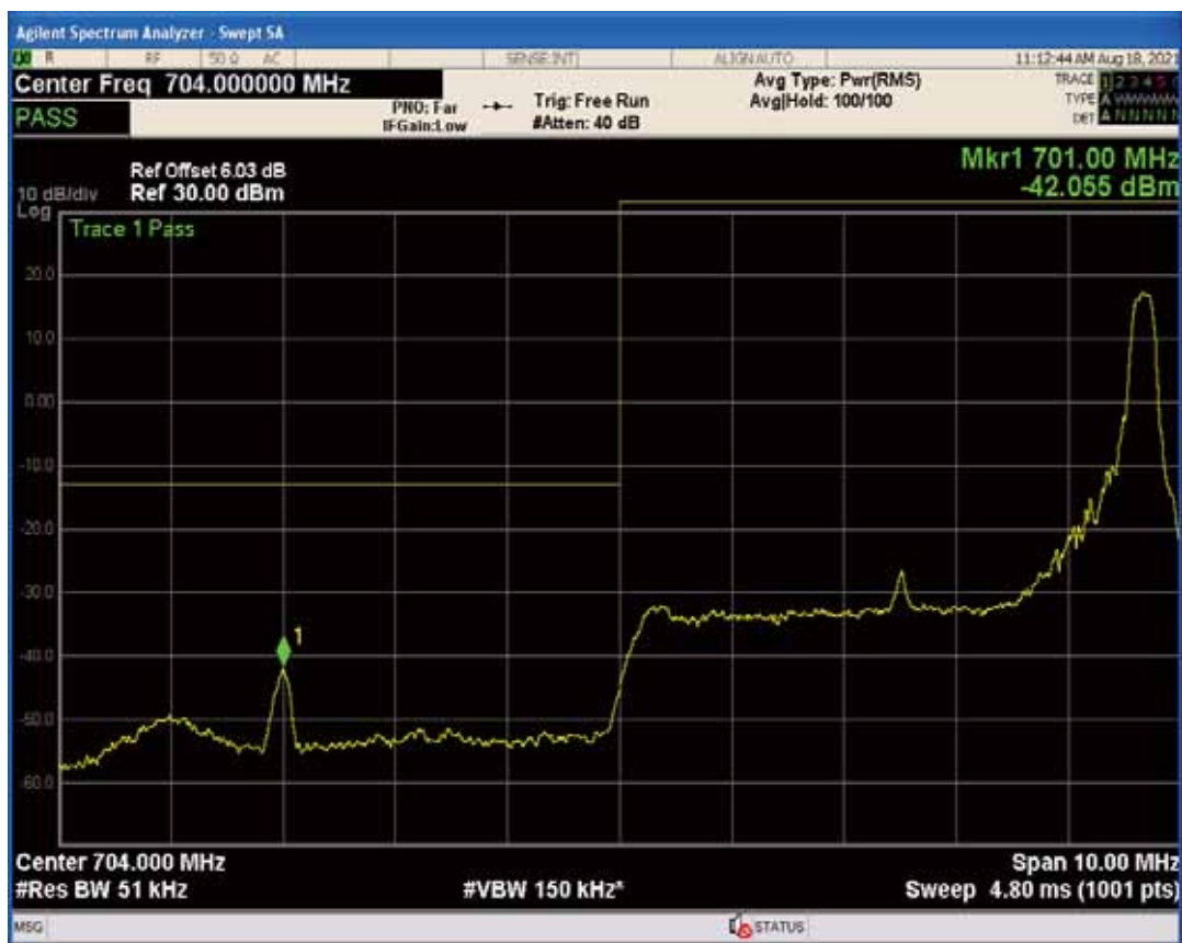
Band17 QAM16 BW=5MHz Channel=23755 RB Size=25 Position=#0
