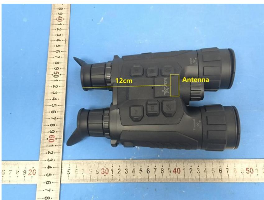
Minimum distance from antenna to eyepiece (Head): 12cm
