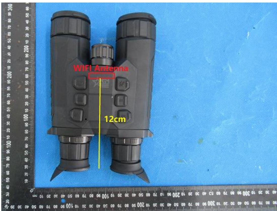
Minimum distance from antenna to eyepiece (Head): 12cm
