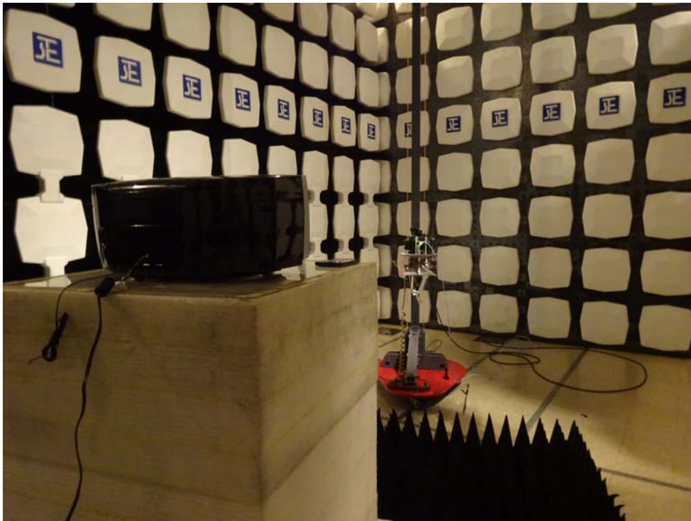
Measurement of Radiated Emission Test Set Up
