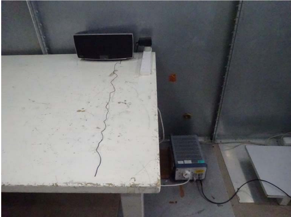
Measurement of Conducted Emission Test Set Up
