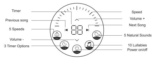
**Power On/Off:** Press button to power on swing. Power light turns green when swing is powered on. Press again to turn off.
