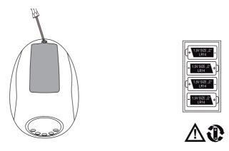
Note:Low battery power may cause product movement to slow, sound and lights to become faint, or product to turn off altogether. If this should happen, use the AC adaptor as a power source or replace the batteries.
