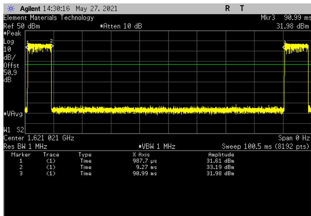
Transmit, DE-QPSK, Mid Ch. 121, 1621.020833 MHz
