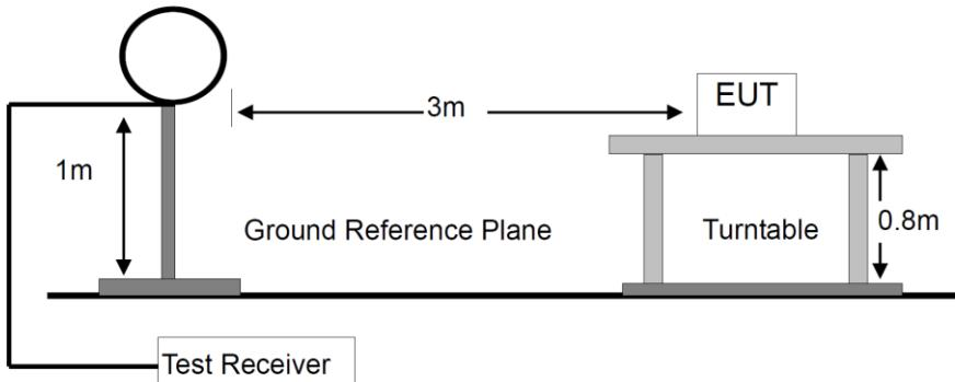
For Radiated Emission 30-1000MHz
