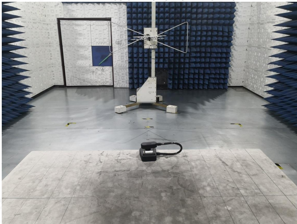
RADIATED EMISSION TEST SETUP ABOVE 1GHZ
