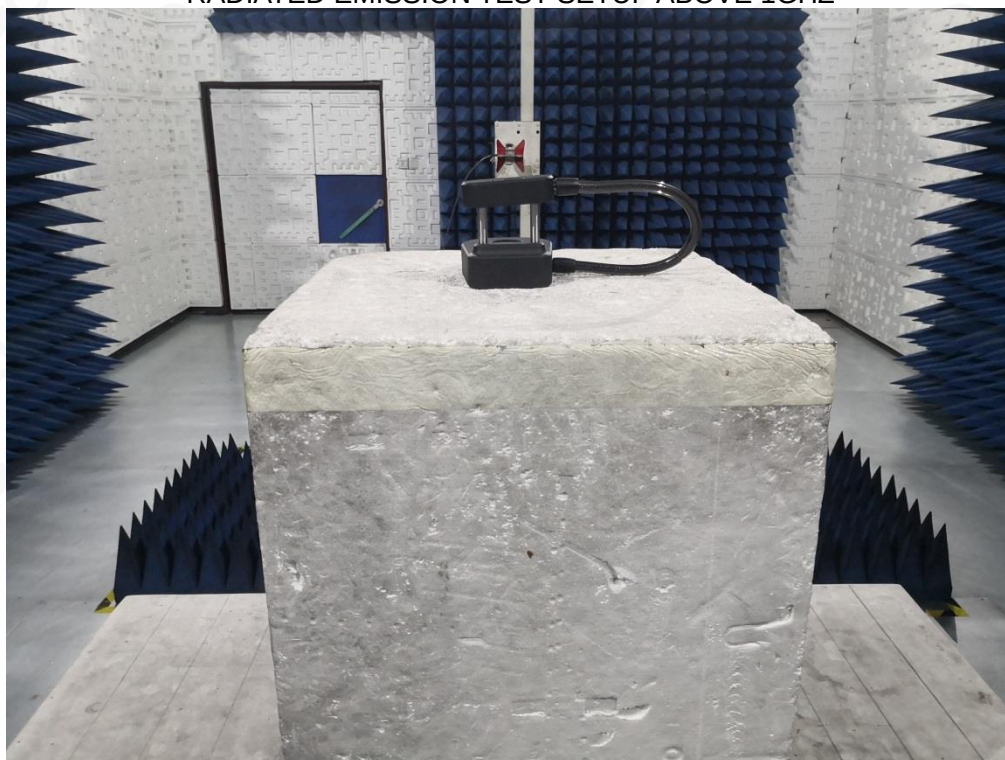
RADIATED EMISSION TEST SETUP ABOVE 1GHZ
