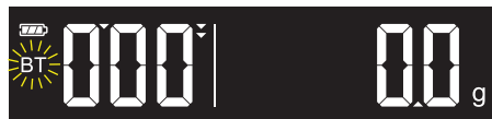
Press "BT" button one time to open Bluetooth, BT mark will flash during the process of connecting.
