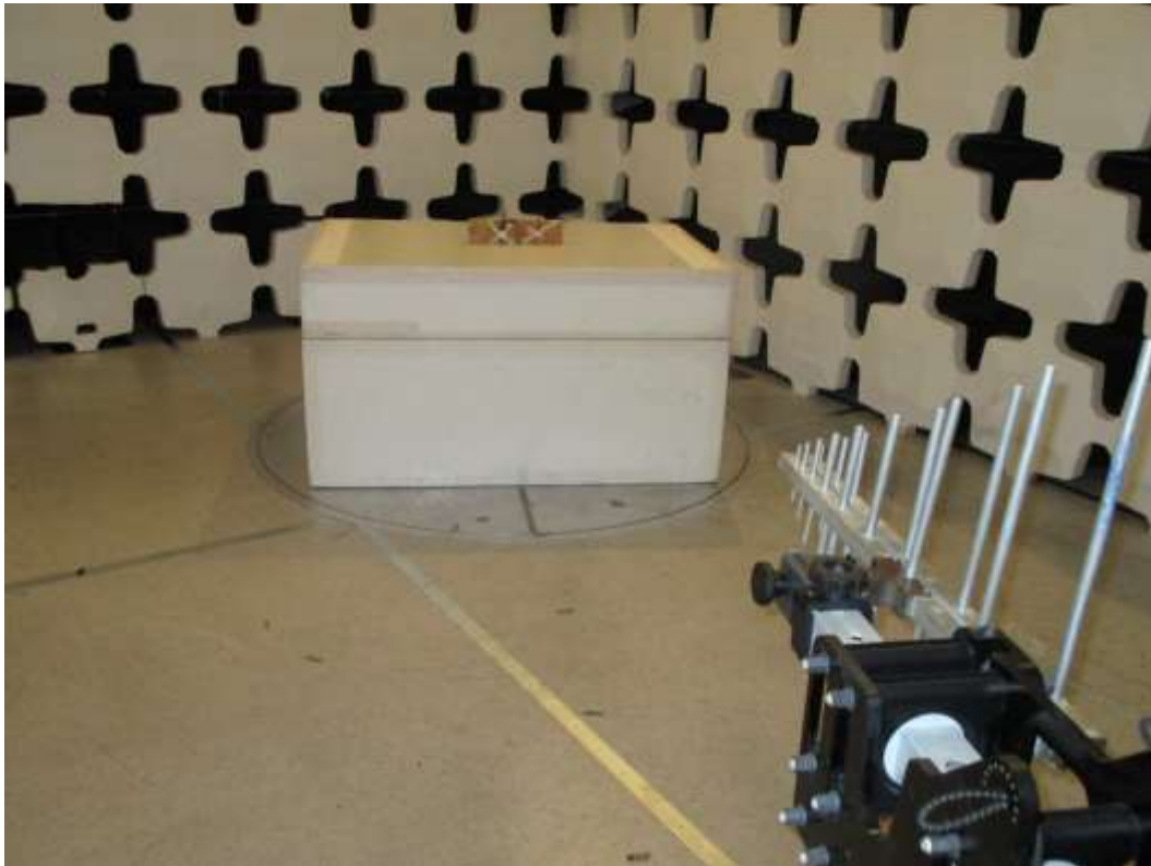
Figure 4. Radiated Emissions Test Configuration (200 - 1000 MHz)
