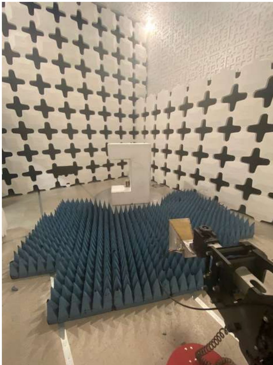
Figure 4. Radiated Emissions Test Configuration (above 1000 MHz, Intentional Emissions)
