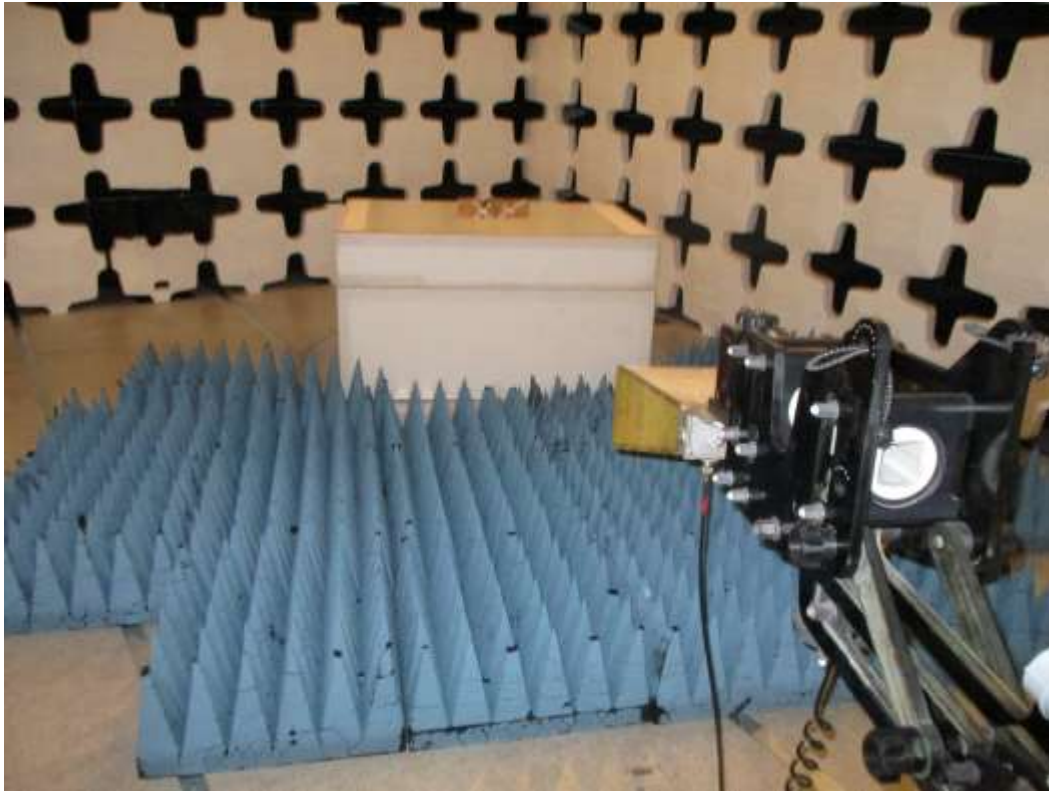
Figure 3. Radiated Emissions Test Configuration (above 1000 MHz, Unintentional Emissions)
