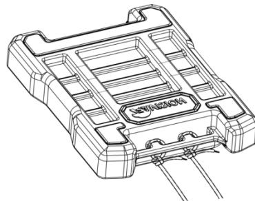
3. Place the ropes and the lifting installation module inside the frame and confirm that the rope length is between 5-10m.
