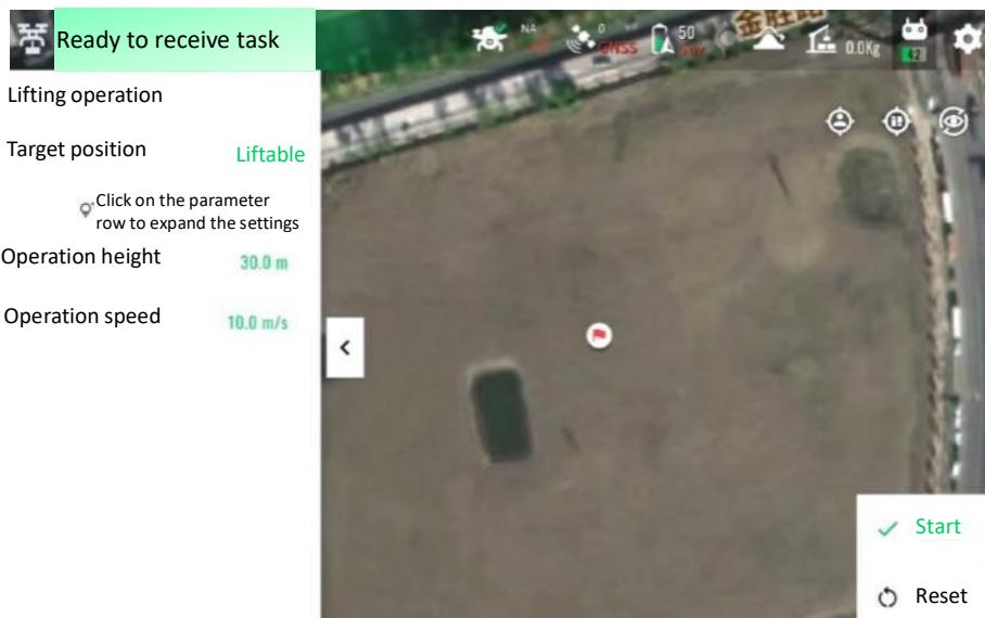
6. After reaching the designated position, hover and lower the height. After hanging the cargo, communicate with the person hanging the cargo. First, raise the height to check whether the weight exceeds the limit when the cargo leaves the ground, and then click "Return".
