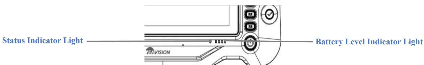
The status indicator lights of the remote controller use lights of three colors with different flashing frequencies to represent different meanings.
