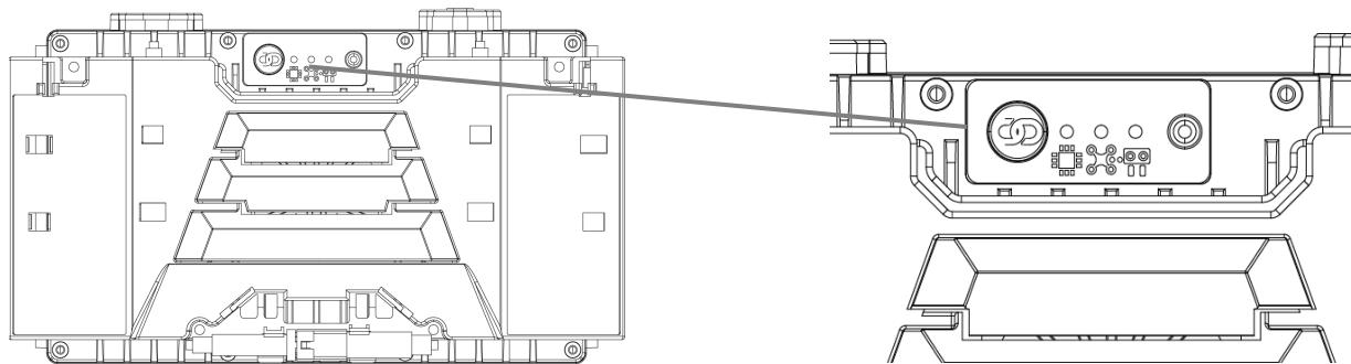
4. Wait for about 30 seconds. When the pairing status indicator light of the remote controller turns green and stays on, and the indicator light of the main controller turns blue and stays on, it indicates that the pairing is successful.
