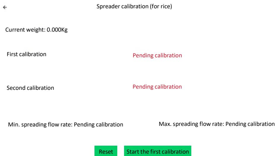
8. After the first calibration is completed, the load cell will automatically calculate the spreading amount. Observe whether the weighed value and the actual spreading amount deviate greatly. If the error is less than 200g, proceed to the next step. If there is a significant weight error, it is recommended to use an electronic scale to weigh the actual spreading weight and re-enter the parameters.
