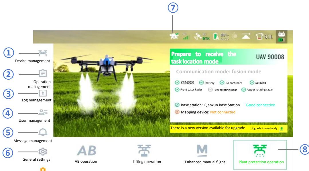
1. Device Management: View the status of the agricultural drone, base station, mapping device, APP version, remote controller, etc.
