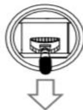
Pull down the throttle to make the agricultural drone land, and then pull the throttle stick to the lowest position and hold it. After 3 seconds, the motor stops.
