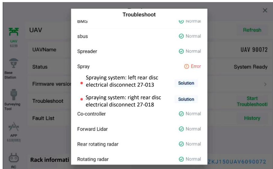
4. Click "Solution" and solve the corresponding fault according to the prompts.
