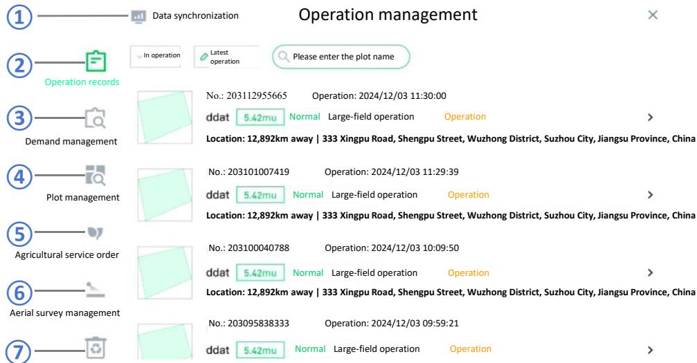
1. **Data Synchronization:** When operating offline, data that cannot be transmitted back to the server is temporarily stored locally. After the remote controller is connected to the network, it can be transmitted back to the server. Click to view information such as plots, tasks, planning, and flight missions.
