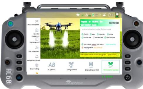
The top-status bar on the home page displays the time, network connection status, and the remaining battery level of the remote controller.
