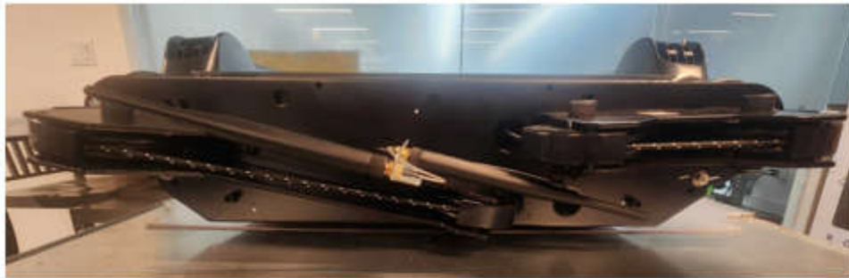
Inside Top with WiFi Dipole Antennas
