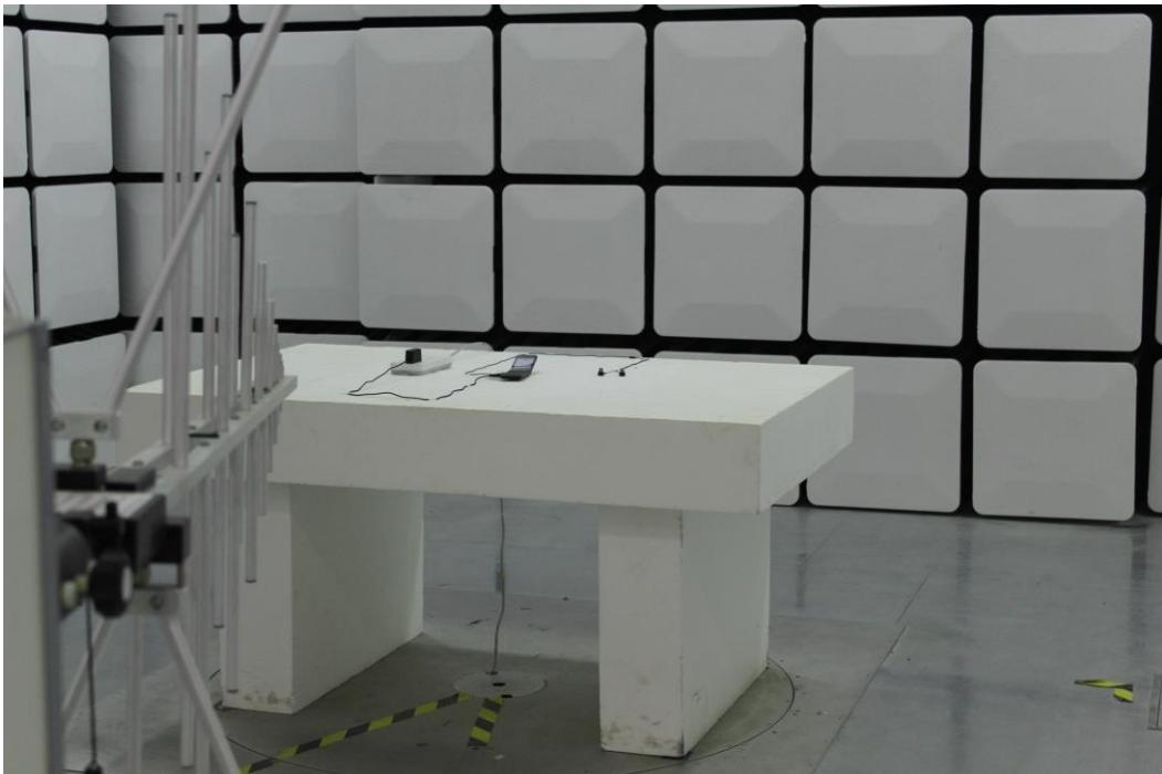
**1.3 Setup for Unwanted Emissions that fall Outside of the Restricted Bands(Radiated) and Unwanted Emissions in the Restricted Bands (Radiated) above 1GHz**
