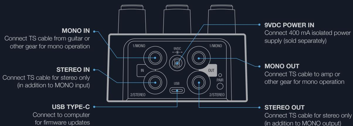
**Power Supply** Isolated 9VDC, center-negative, 400 mA minimum, 2.1x5.5 mm barrel connector (sold separately)
