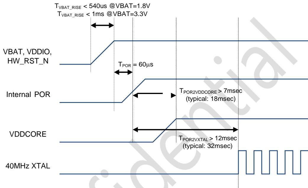
Boot up by HW\_RST\_N pin, power on timing is shown in below figure.
