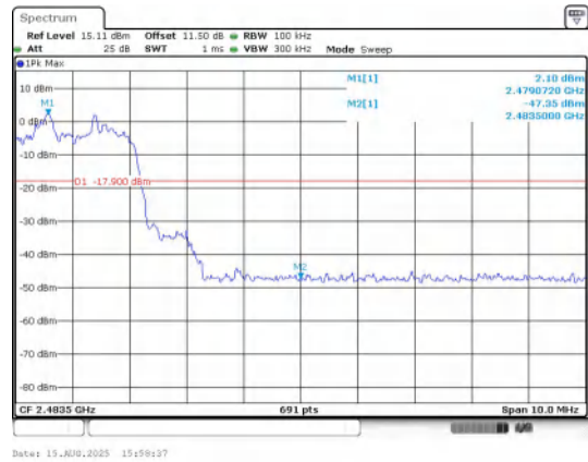
Out Of Band Emission(Right) \pi/4 DQPSK_2-DH5_Channel Hopping
