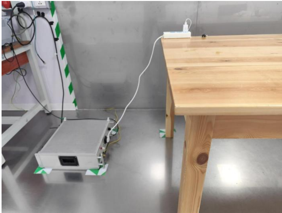
Conducted Emission at AC power line
