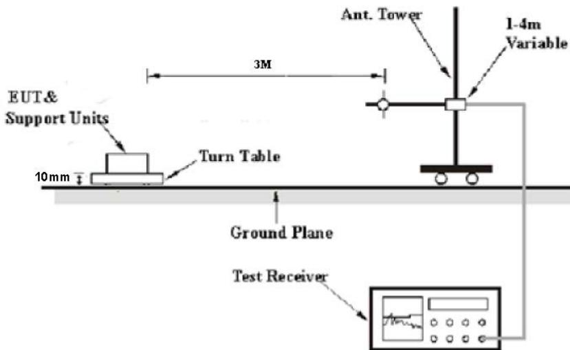
The radiated emission tests were performed in the 3 meters chamber test site, using the setup accordance with the ANSI C63.10-2013. The specification used was the FCC 15.209 and FCC 15.205 limits.
