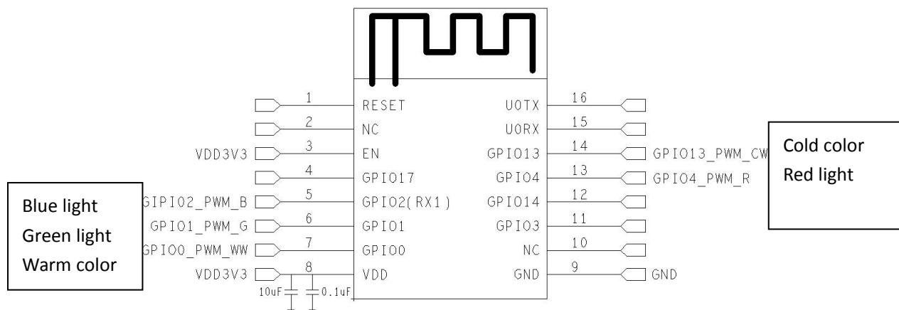
The module can support five PWM channels, and the user can select the corresponding PWM interface according to the actual product situation. The corresponding color can also modify the customized firmware according to the actual needs;
