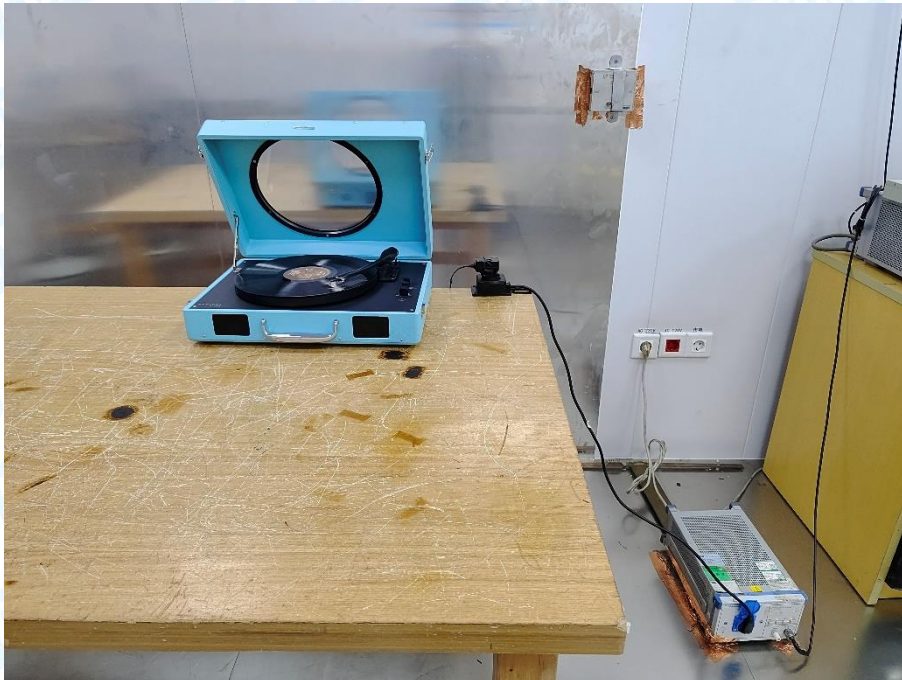
Photo of Setup for Radiated Emission (30MHz~1GHz)
