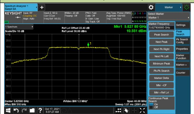
802.11ac-VHT40 Power Spectral Density - Ant 1
