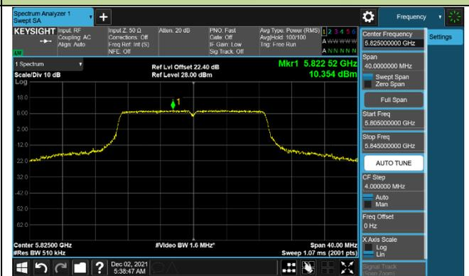
802.11ac-VHT40 Power Spectral Density – Ant 1
