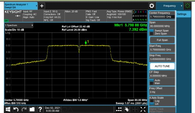
802.11ac-VHT80 Power Spectral Density – Ant 1
