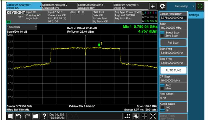
802.11ac-VHT160 Power Spectral Density – Ant 1
