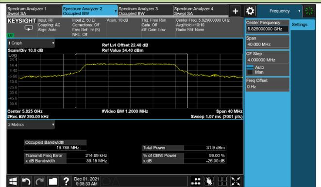
802.11ac-VHT20 26dB Bandwidth & 99% Bandwidth
