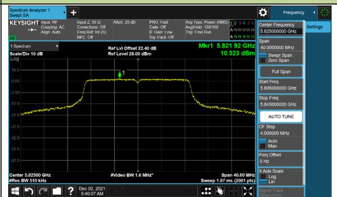
802.11ac-VHT40 Power Spectral Density – Ant 0
