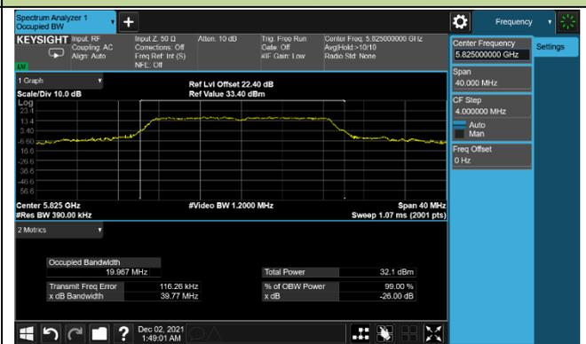
802.11ac-VHT40 26dB Bandwidth & 99% Bandwidth
