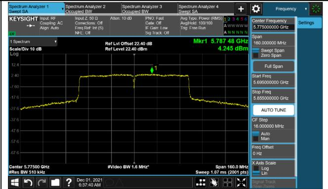
802.11ac-VHT160 Power Spectral Density – Ant 0
