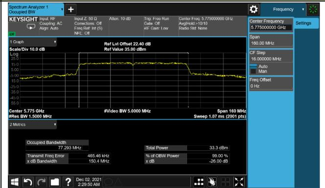
802.11ac-VHT160 26dB Bandwidth & 99% Bandwidth
