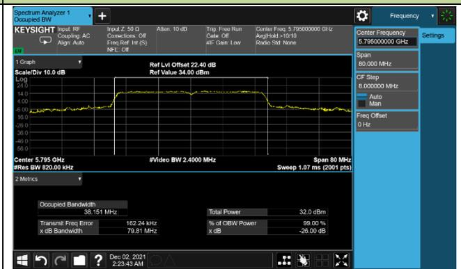
802.11ac-VHT80 26dB Bandwidth & 99% Bandwidth
