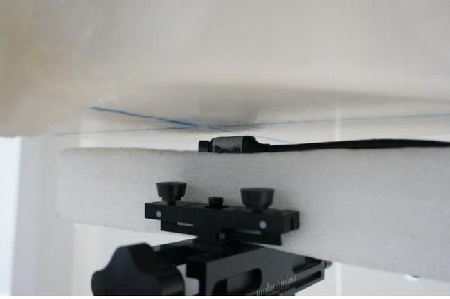
A photograph showing a back view of the test setup. The black device is resting on a white foam block. A blue laser line is visible, intersecting the device and the foam. The background is a plain white surface. |
