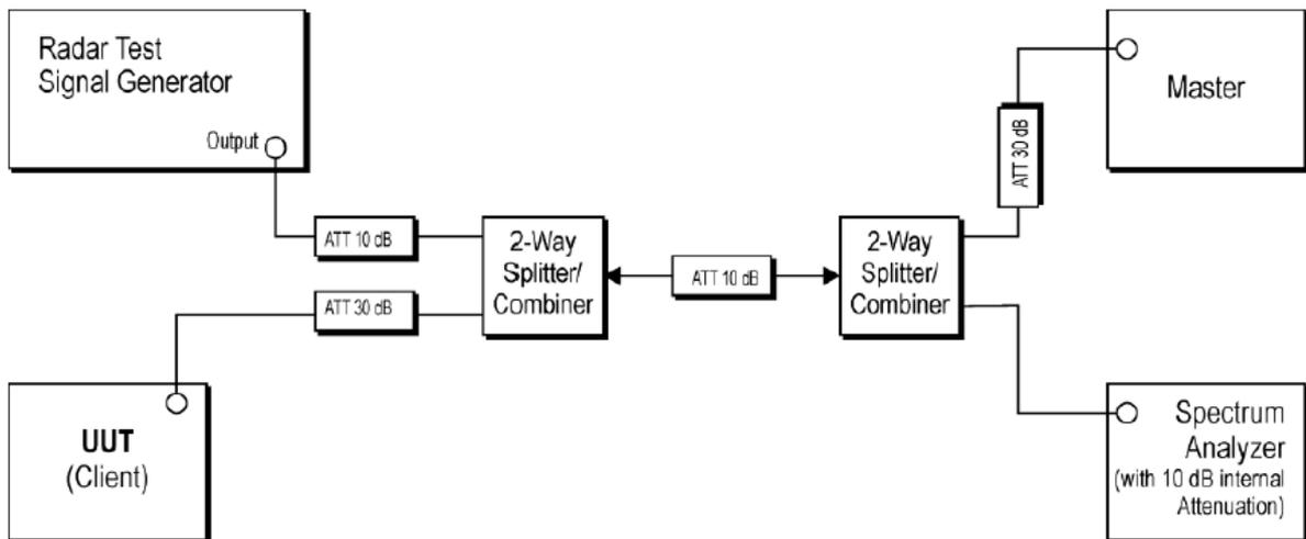
Radar Test Waveforms are injected into the Master.
