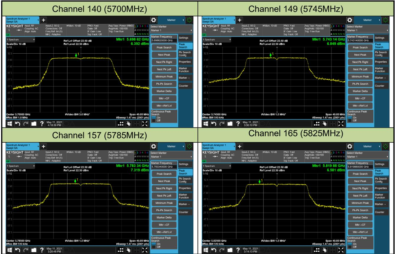
802.11ac-VHT40 Power Spectral Density – Ant 1/Ant 0 + 1
