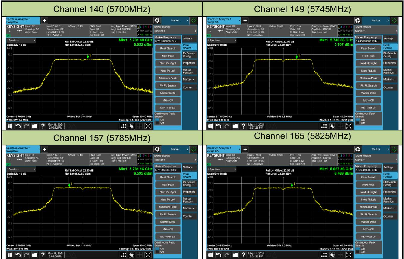
802.11ac-VHT20 Power Spectral Density – Ant 1/Ant 0 + 1
