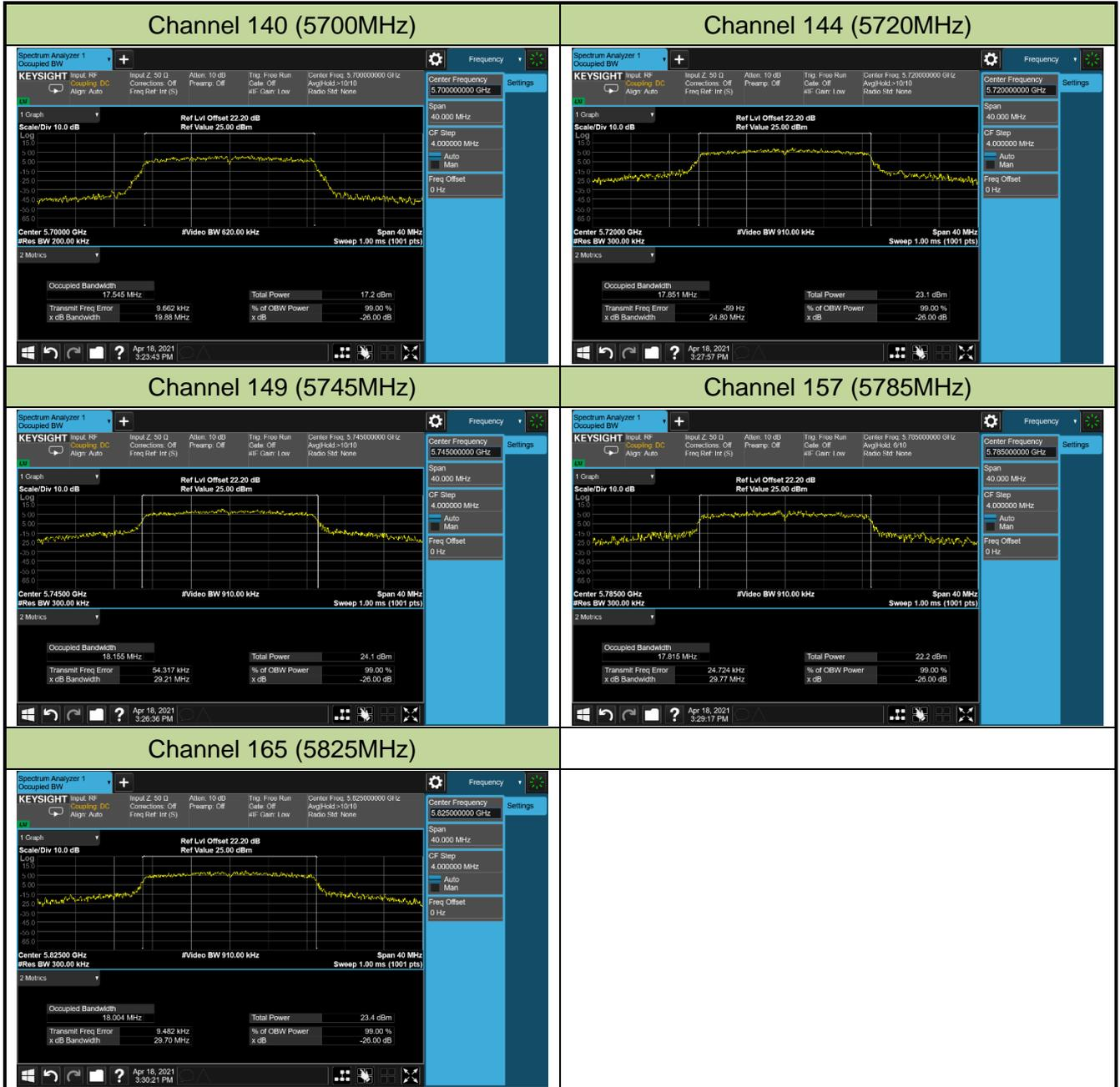
802.11ac-VHT40 26dB Bandwidth & 99% Bandwidth
