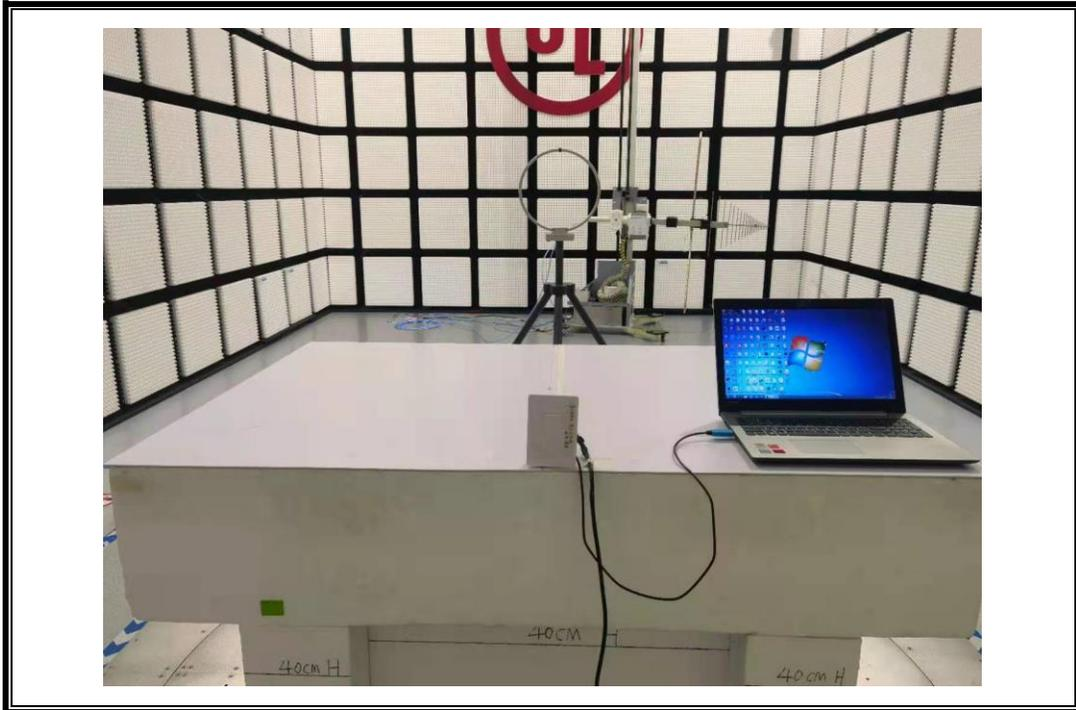
RADIATED RF MEASUREMENT SETUP (Above 1G )
