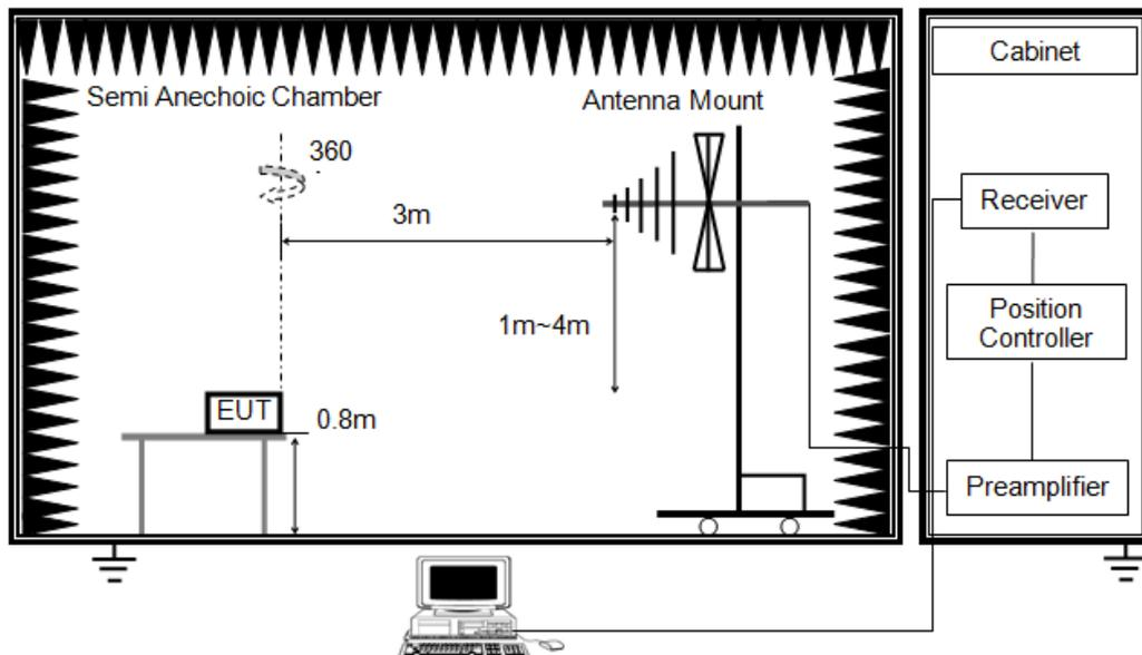
1. The EUT was arranged to its worst case and then turntable (from 0 degree to 360 degrees) to find the maximum reading. A pre-amp and a high pass filter are used for the test in order to get better signal level.
