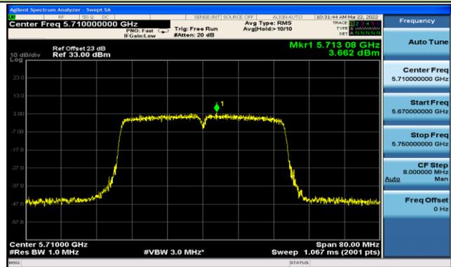
802.11ac-VHT80 Power Spectral Density - Ant 3 / Ant 0 + 1 + 2 + 3\_N<sub>SS</sub> = 4
