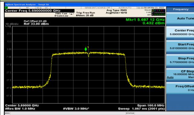
802.11ac-VHT160 Power Spectral Density - Ant 3 / Ant 0 + 1 + 2+ 3\_Nss = 4
