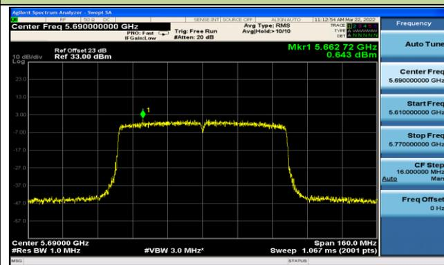
802.11ac-VHT160 Power Spectral Density - Ant 2 / Ant 0 + 1 + 2+ 3\_Nss = 4
