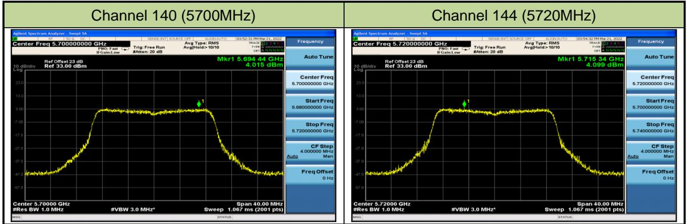
802.11ac-VHT40 Power Spectral Density - Ant 3 / Ant 0 + 1 + 2+ 3\_N<sub>SS</sub> = 4
