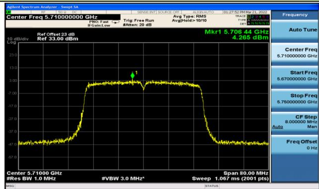
802.11ac-VHT80 Power Spectral Density - Ant 2 / Ant 0 + 1 + 2 + 3\_N<sub>SS</sub> = 4
