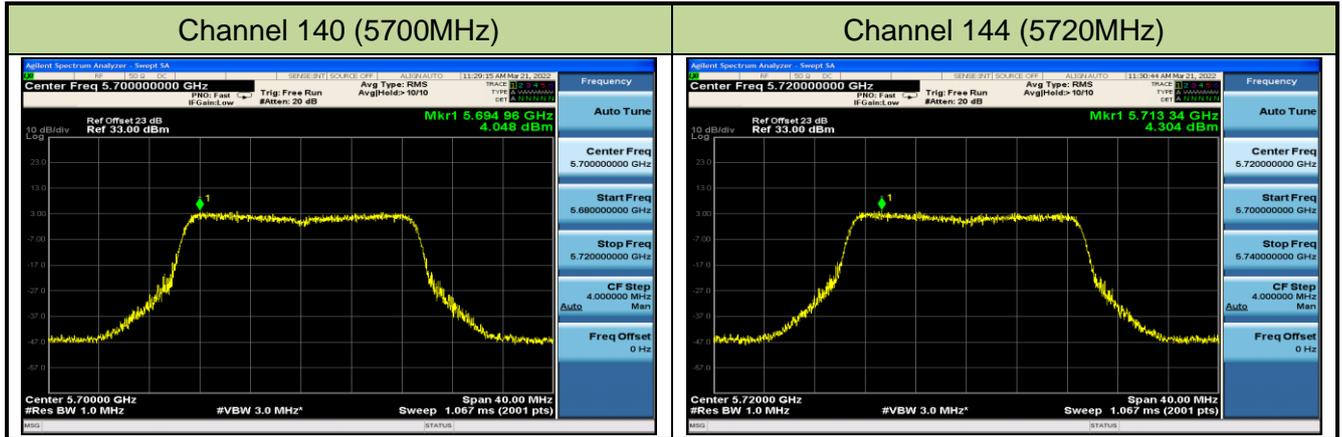
802.11ac-VHT40 Power Spectral Density - Ant 2 / Ant 0 + 1 + 2+ 3\_N<sub>SS</sub> = 4
