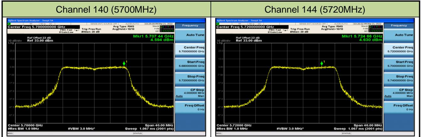
802.11ac-VHT20 Power Spectral Density - Ant 3 / Ant 0 + 1 + 2+ 3\_N<sub>SS</sub> = 4
