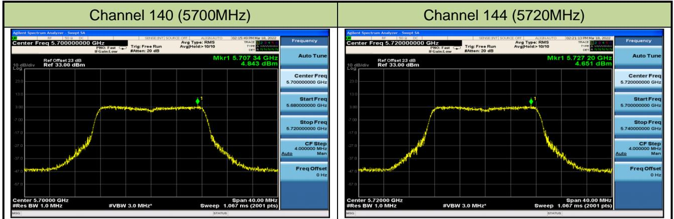
802.11ac-VHT20 Power Spectral Density - Ant 0 / Ant 0 + 1 + 2+ 3\_NSS4
