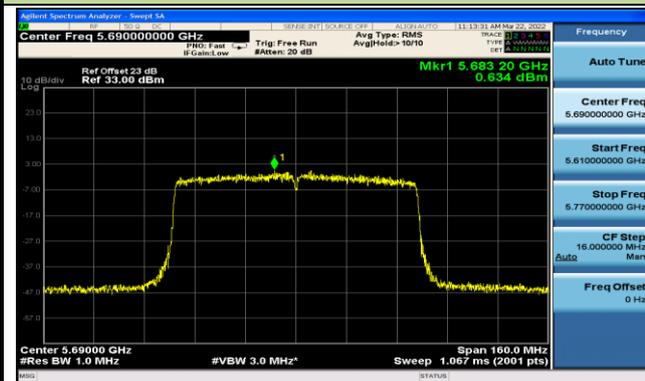
802.11ac-VHT160 Power Spectral Density - Ant 0 / Ant 0 + 1 + 2+ 3\_NSS4
