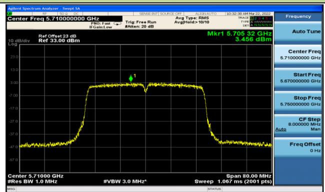
802.11ac-VHT80 Power Spectral Density - Ant 0 / Ant 0 + 1 + 2+ 3\_NSS4
