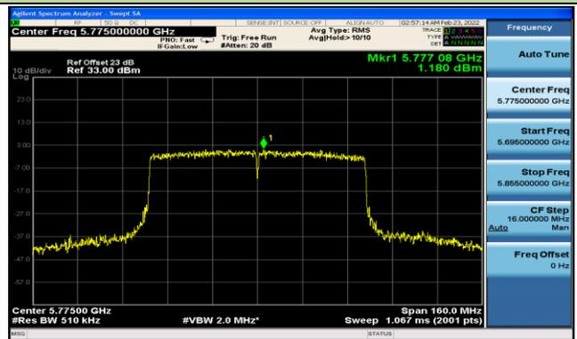
802.11ac-VHT160 Power Spectral Density - Ant 2
