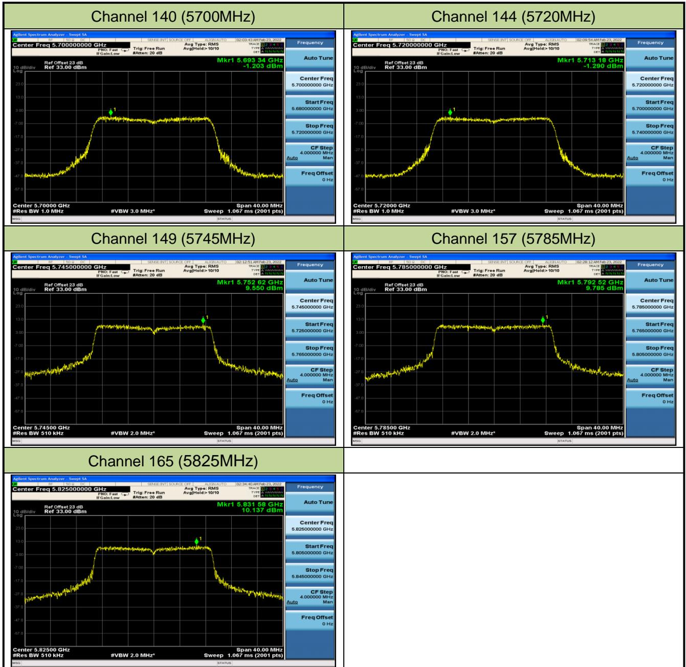
802.11ac-VHT40 Power Spectral Density - Ant 2
