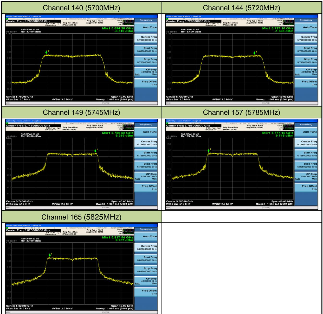
802.11ac-VHT20 Power Spectral Density - Ant 2
