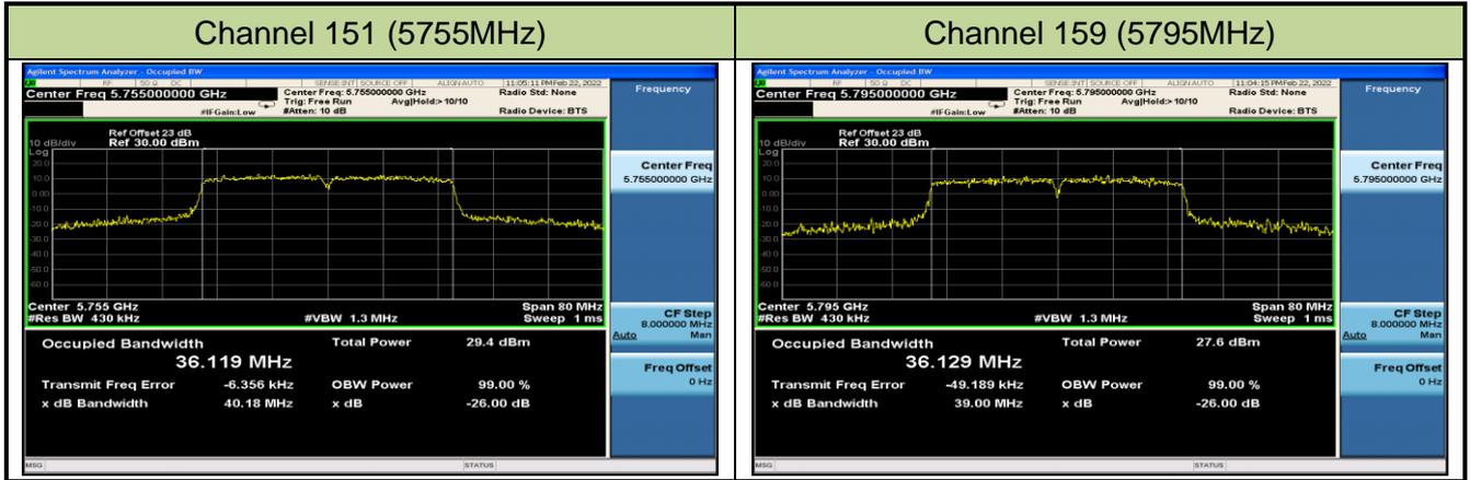
802.11ac-VHT80 26dB Bandwidth & 99% Bandwidth
