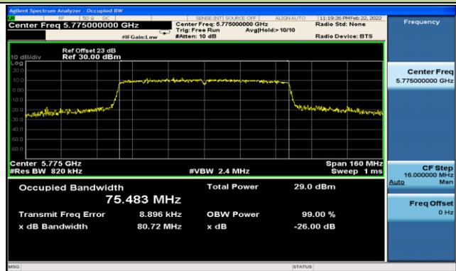
802.11ac-VHT160 26dB Bandwidth & 99% Bandwidth
