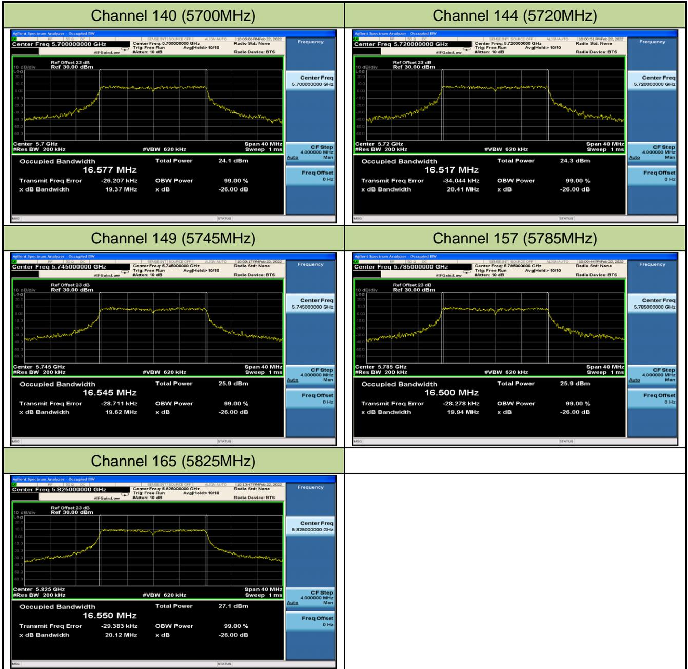
802.11ac-VHT20 26dB Bandwidth & 99% Bandwidth
