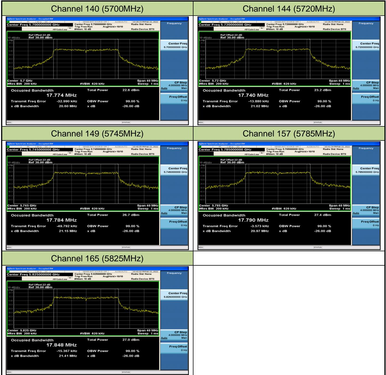
802.11ac-VHT40 26dB Bandwidth & 99% Bandwidth
