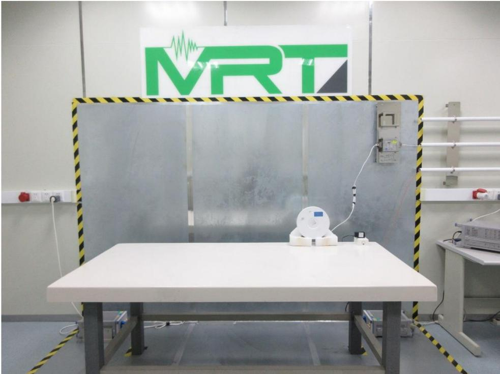
Description: Back View of Conducted Emission Test Setup - 0.15MHz ~ 30MHz
