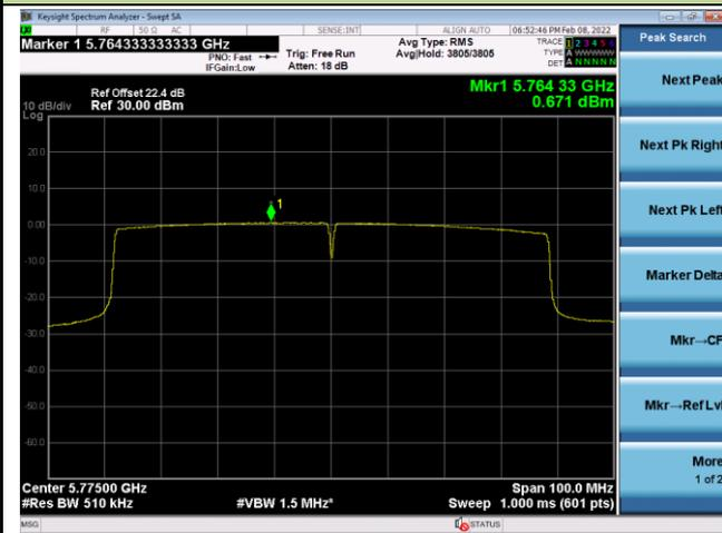
802.11ac-VHT160 Power Spectral Density - Ant 1
