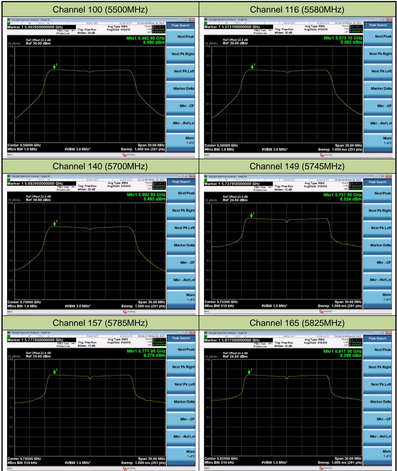
802.11ac-VHT20 Power Spectral Density - Ant 1
