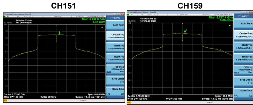
Test Mode UNII-3\_TX AX(HE40) Mode\_Ant. 2
