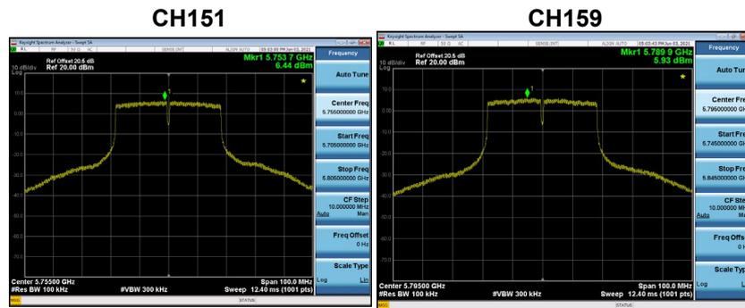
Test Mode UNII-3\_TX AC(VHT40) Mode\_Total
