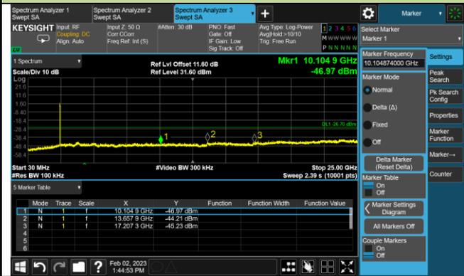
**A.6 Radiated Spurious Emission Test Result**
