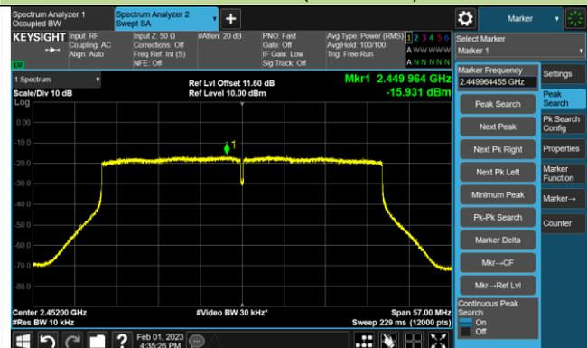
**A.5 Conducted Band Edge and Out-of-Band Emissions Test Result**
