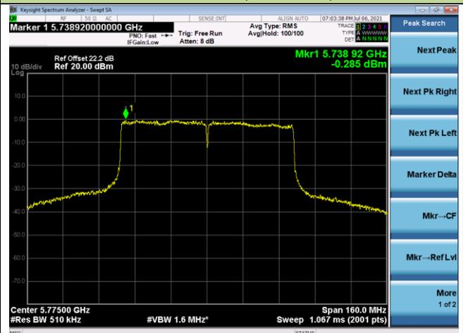
802.11ac-VHT160 Power Spectral Density – Ant 2
