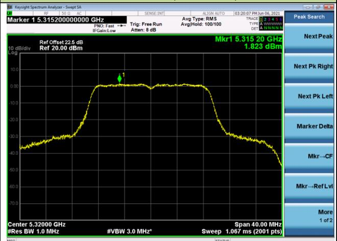
802.11ac-VHT20Power Spectral Density – Ant 2
