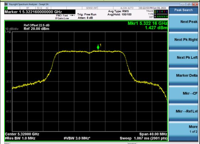
802.11ac-VHT20Power Spectral Density – Ant 0
