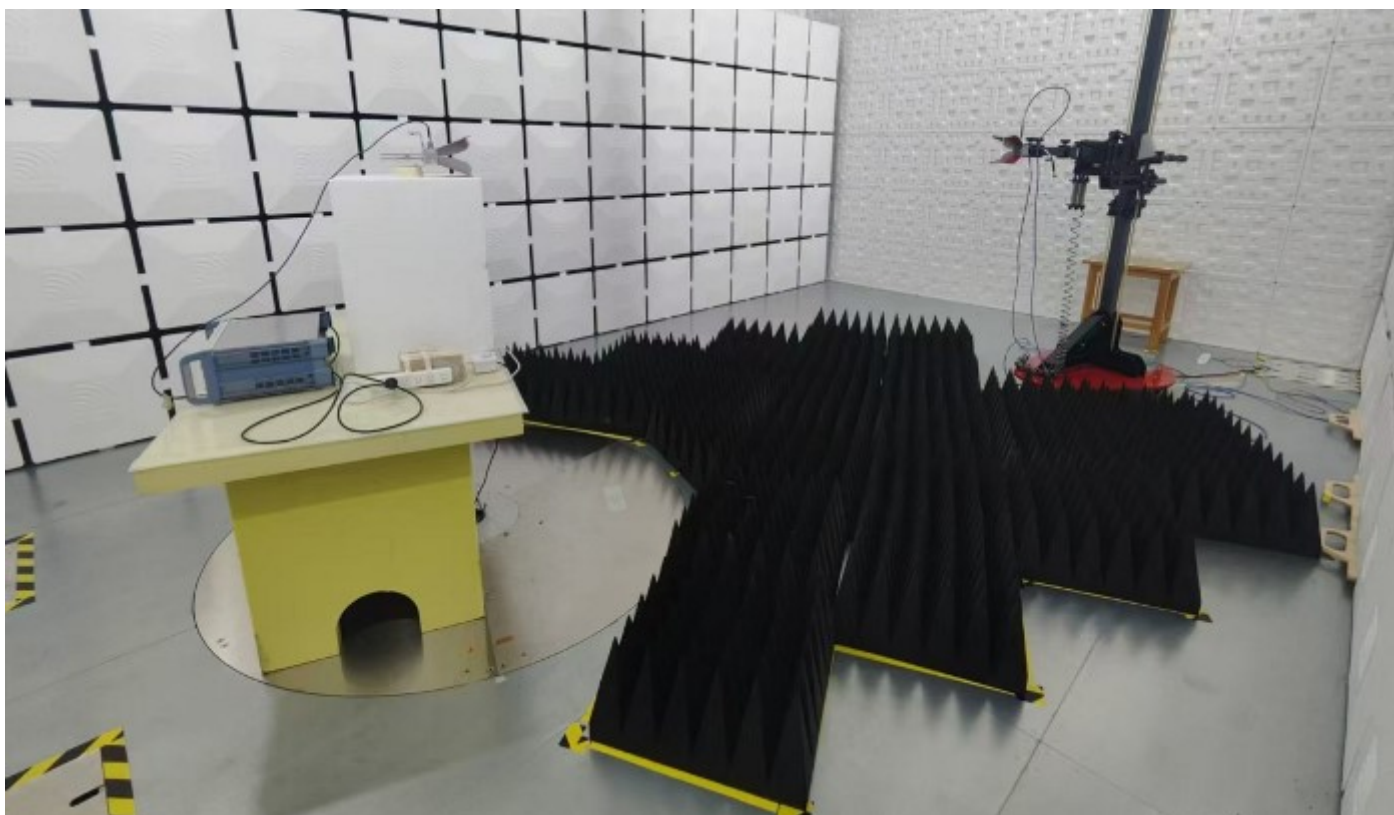
Figure 19 Contention-based protocol test setup photo, radiated method, power measurement
