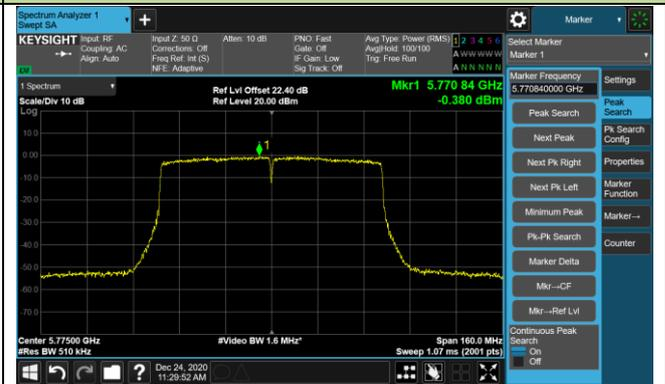
802.11ac-VHT160 Power Spectral Density - Ant 1
