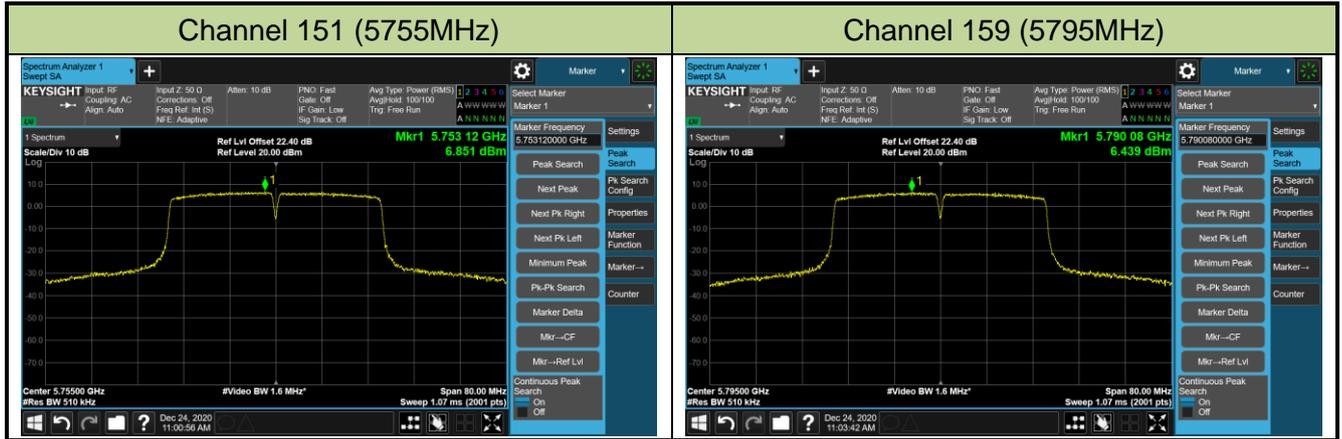
802.11ac-VHT80 Power Spectral Density - Ant 1
