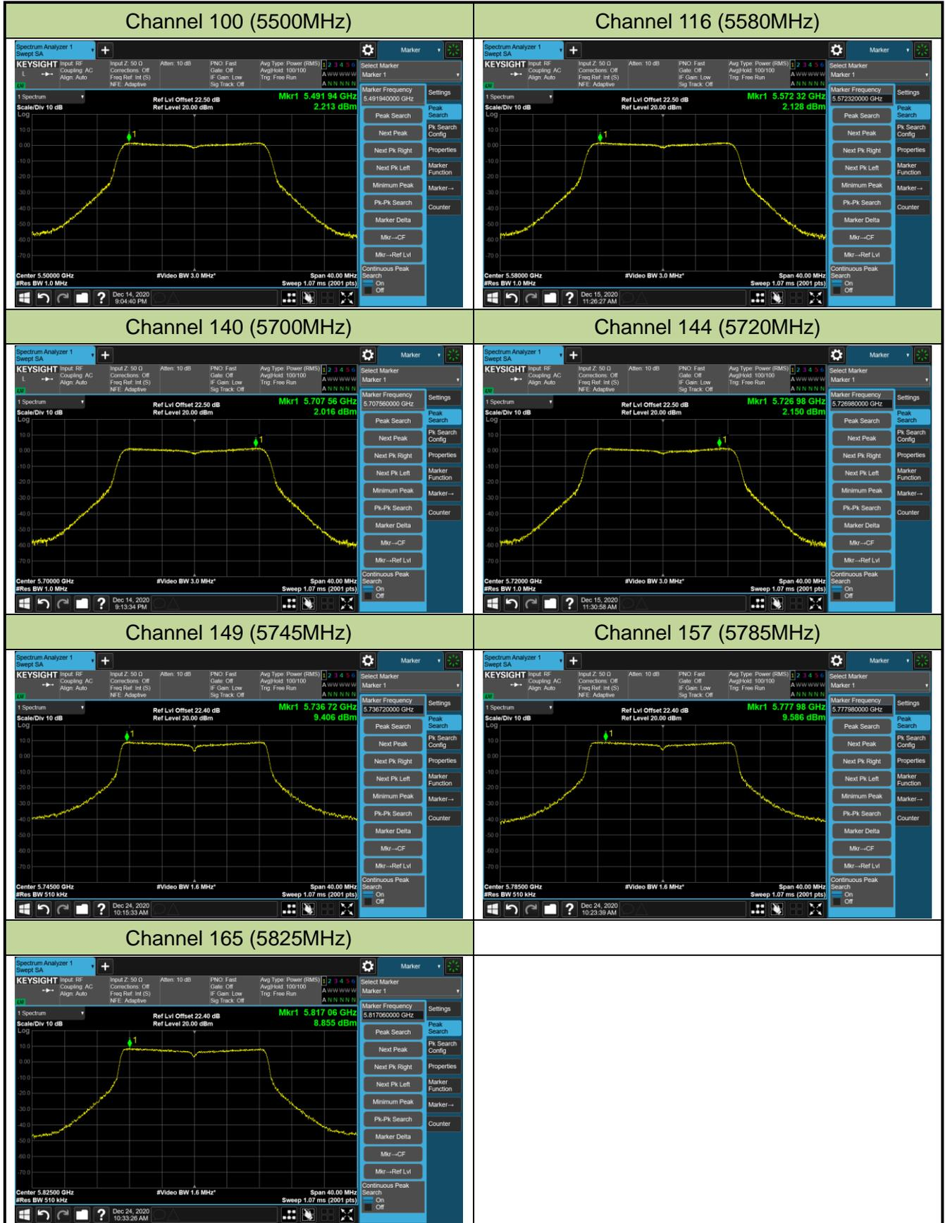
802.11ac-VHT40 Power Spectral Density - Ant 1
