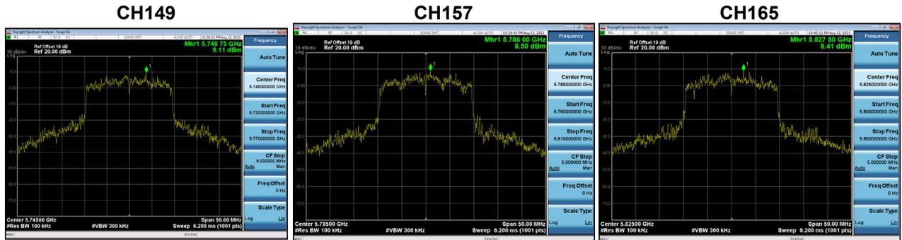
Test Mode UNII-3\_TX AX(HE20) Mode\_Ant. 2
