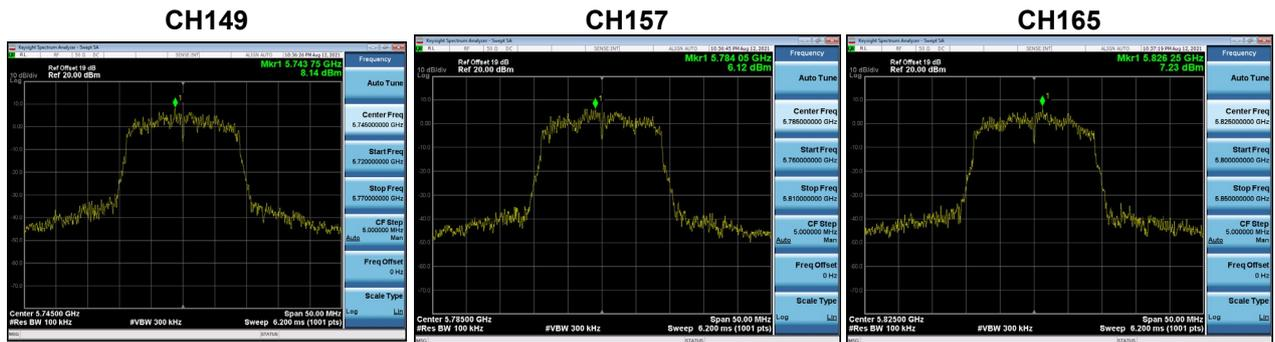
Test Mode UNII-3\_TX AC(VHT20) Mode\_Ant. 2
