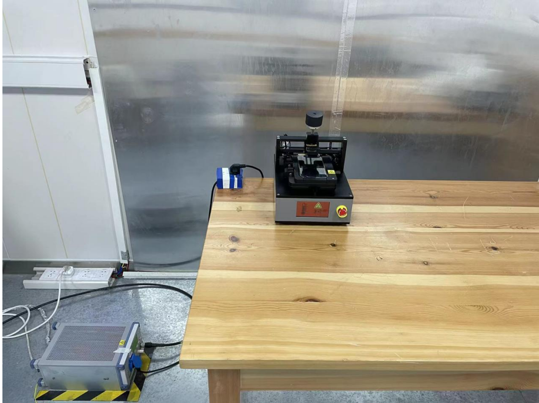
Conducted emission test setup
